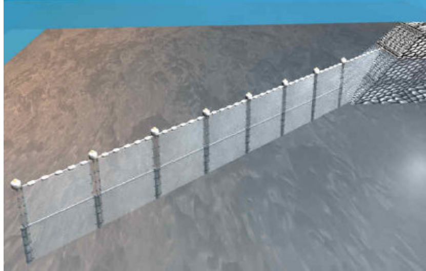
Figure 5 Diagram of Net System with Typical Net Panels and Groin Connection
