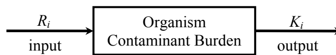
Figure 1 Schematic of a single compartment contaminant mass balance model with multiple inputs and outputs from a single compartment.
