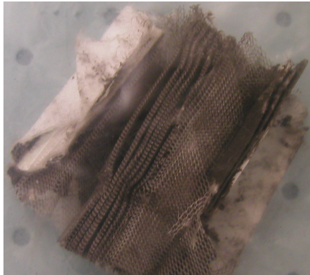
Figure 3: Sample of a Fueling Machine Filter Material
