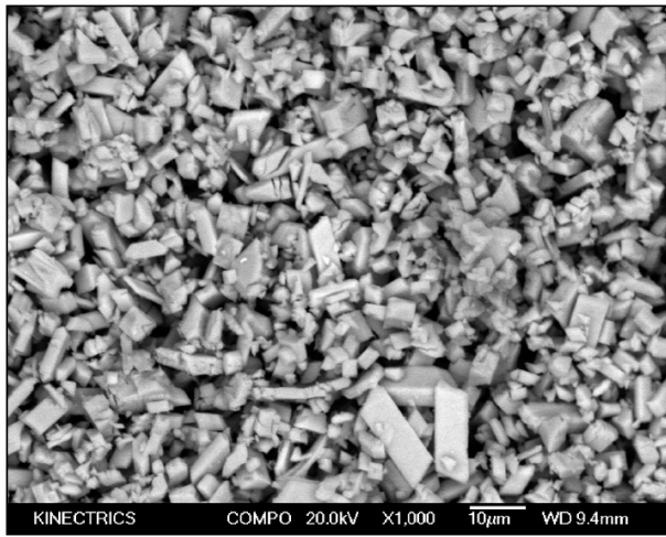
Figure 4 Gadolinium oxalate deposit removed from valve internal
