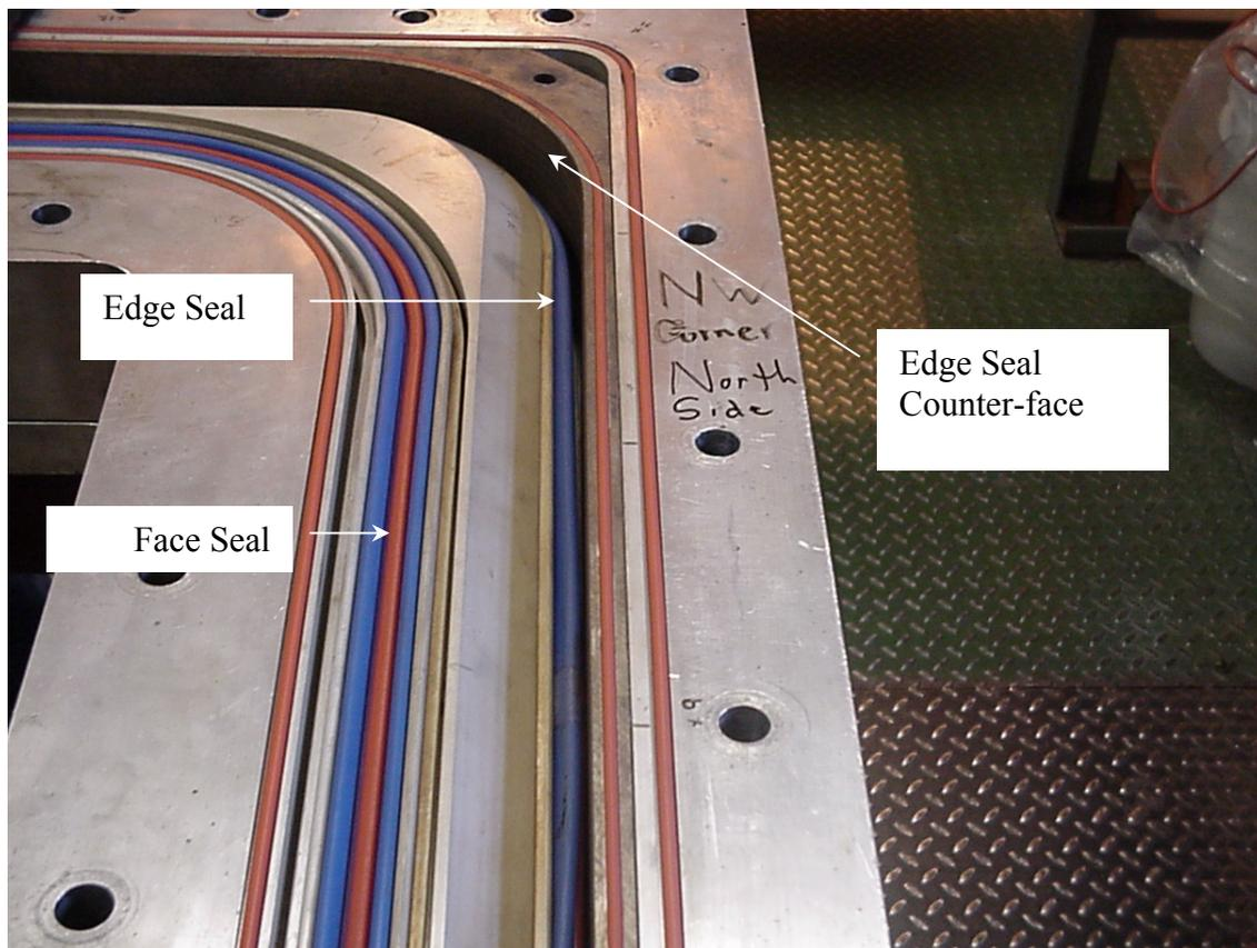
Figure 6: Edge Seal Shown Partially Un-seated Following a Maximum Cross-seal Pressure Test
