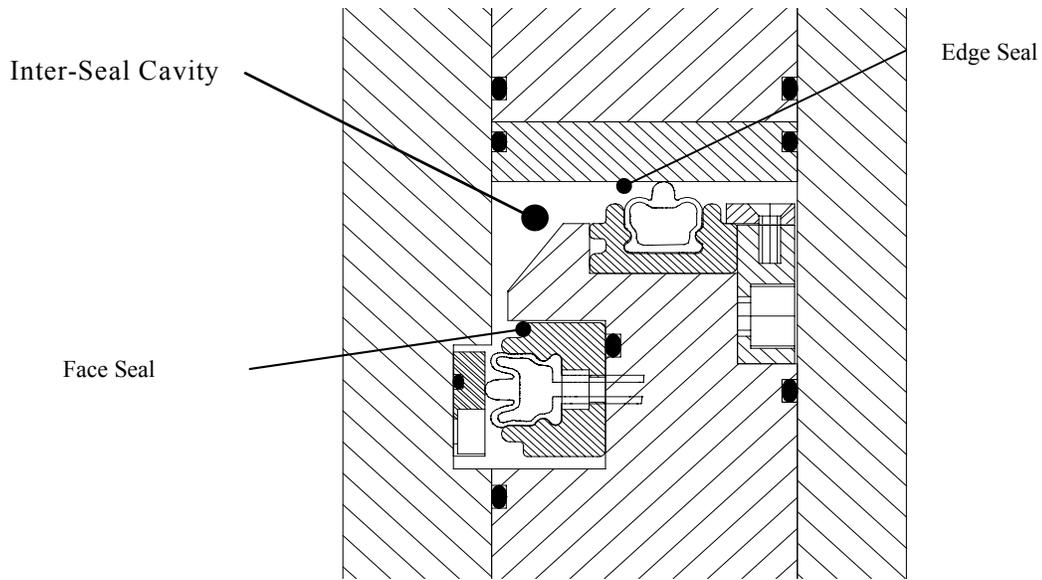
Figure 5: Test Rig Cross-Section Showing Sealing Configurations and Testing Arrangement
