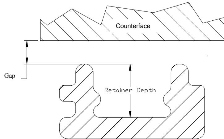
Figure 1: Gap Definition Shown on a Half-Section of a Retainer for Inflatable Door Seals in CANDU 6 Plants
