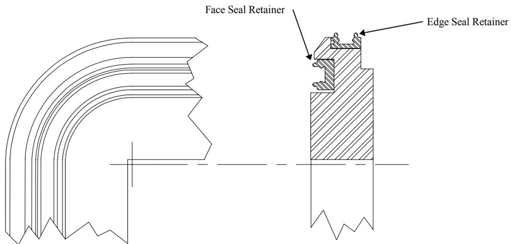
Figure 2: A Cross-Section of the Door Seal EQ Test Rig Showing Edge and Face-Sealing Configurations
