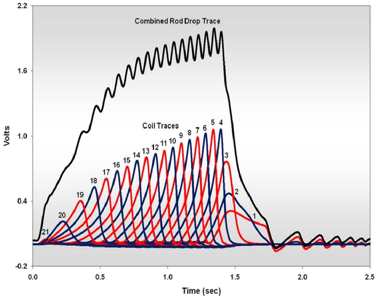
Figure 9 DRPI data during rod drop from step 226 to step 0.
