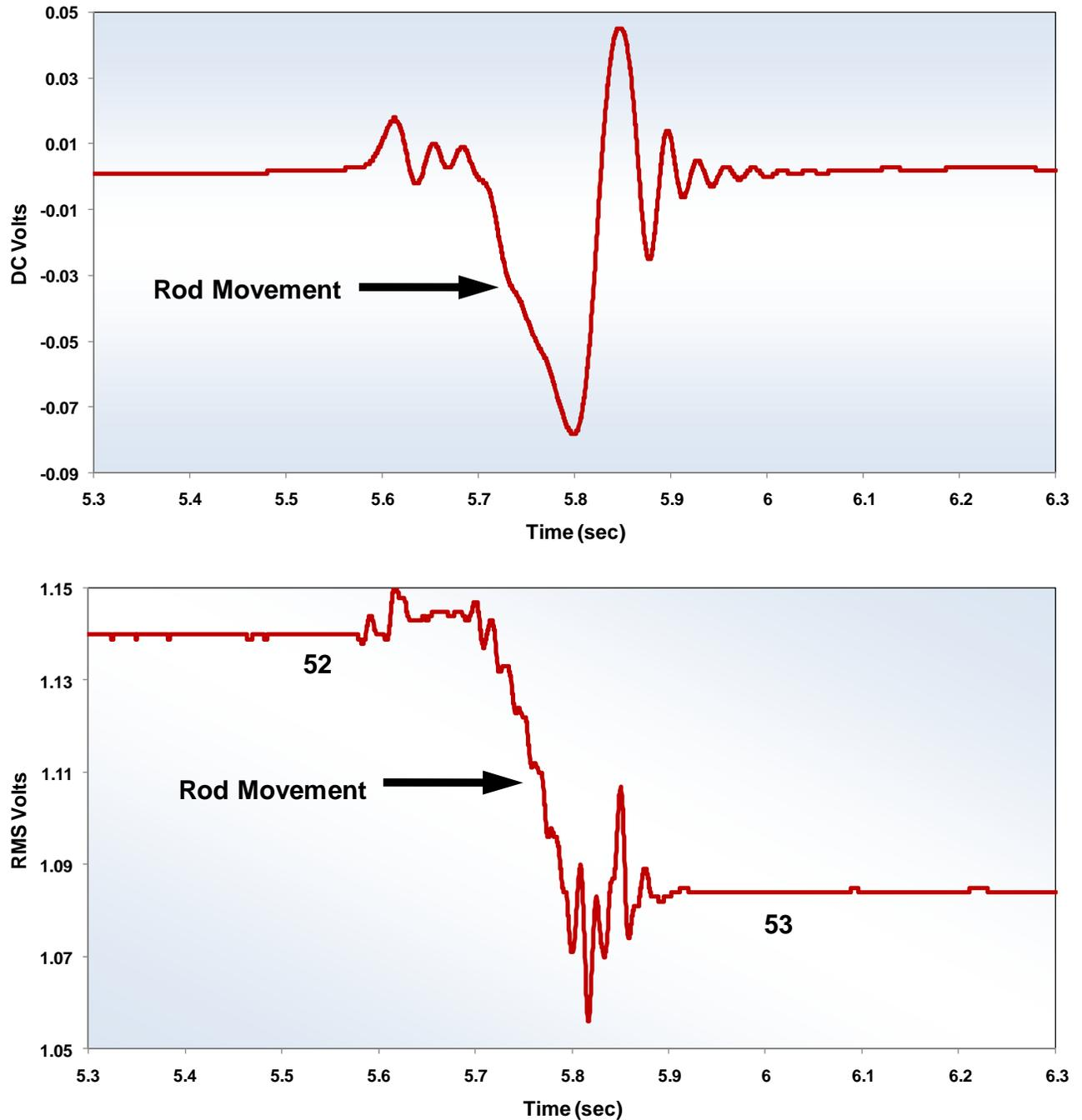
Figure 8 DRPI data during rod withdraw step 52 to step 53.
