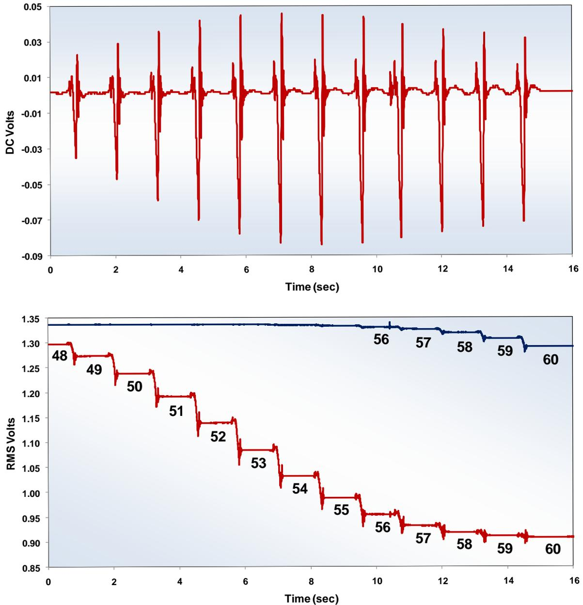
Figure 7 DRPI data during rod withdraw 48-60 steps.
