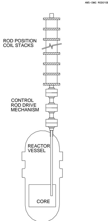
Figure 1 Location of rod position indication coil stacks.
