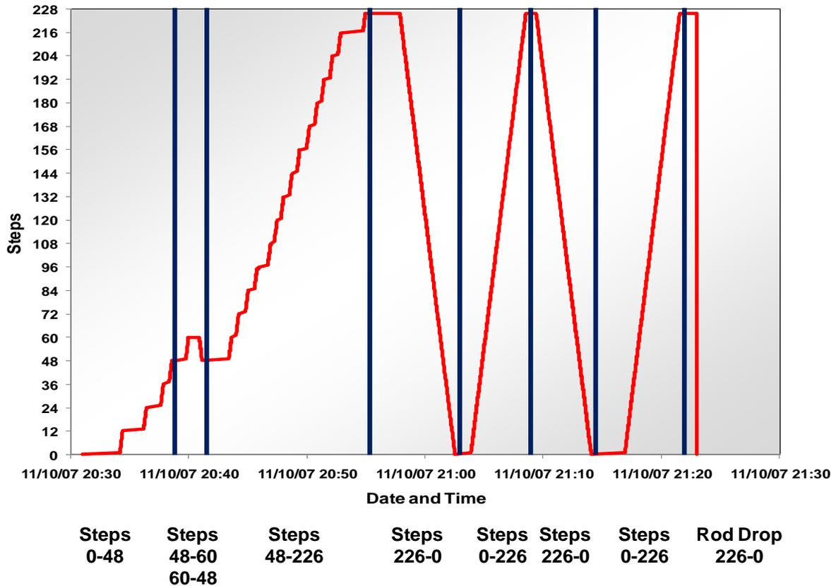
Figure 5 Control Bank D test sequence.
