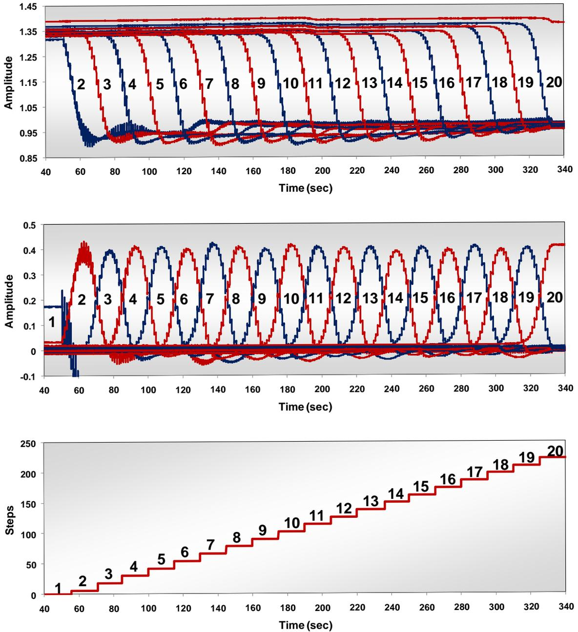
Figure 6 Position measurement during rod withdraw 226 steps.
