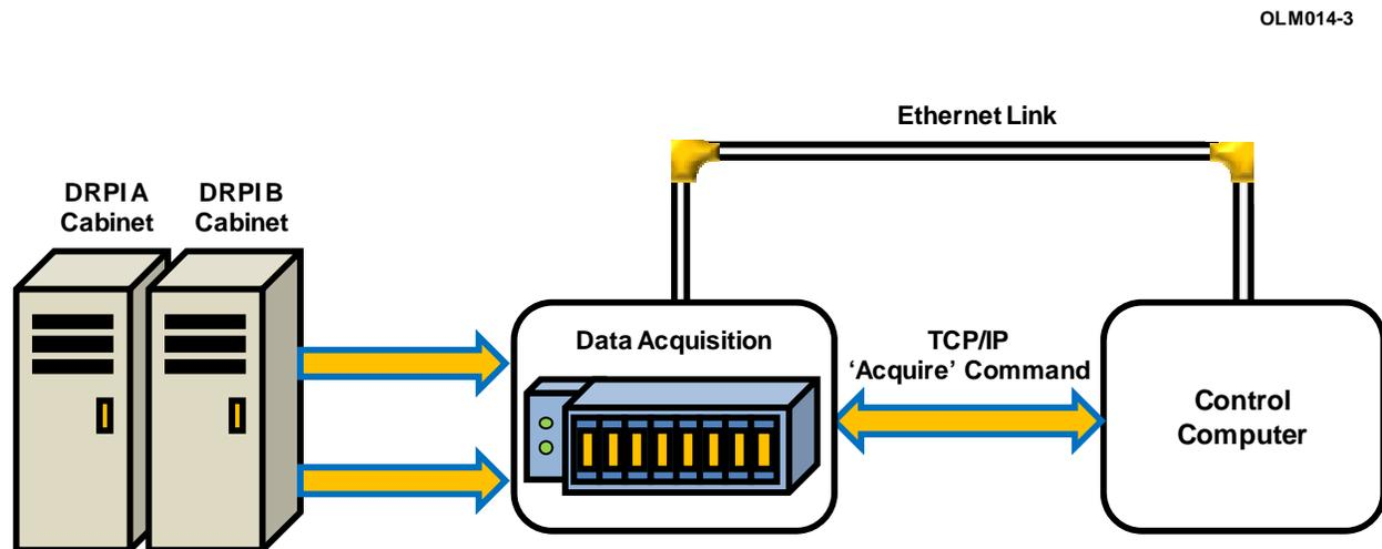
Figure 4 Test equipment setup for prototype system test.
