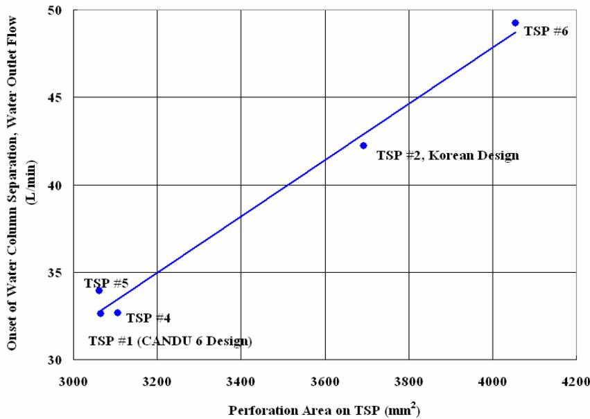
Figure 9: Effect of Perforation Area on OWCS
