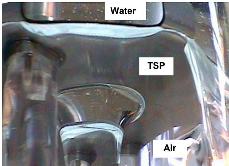
Figure 6: Complete Water Column Separation
