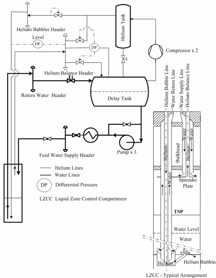
Figure 2: Simplified Schematic of LZCS
