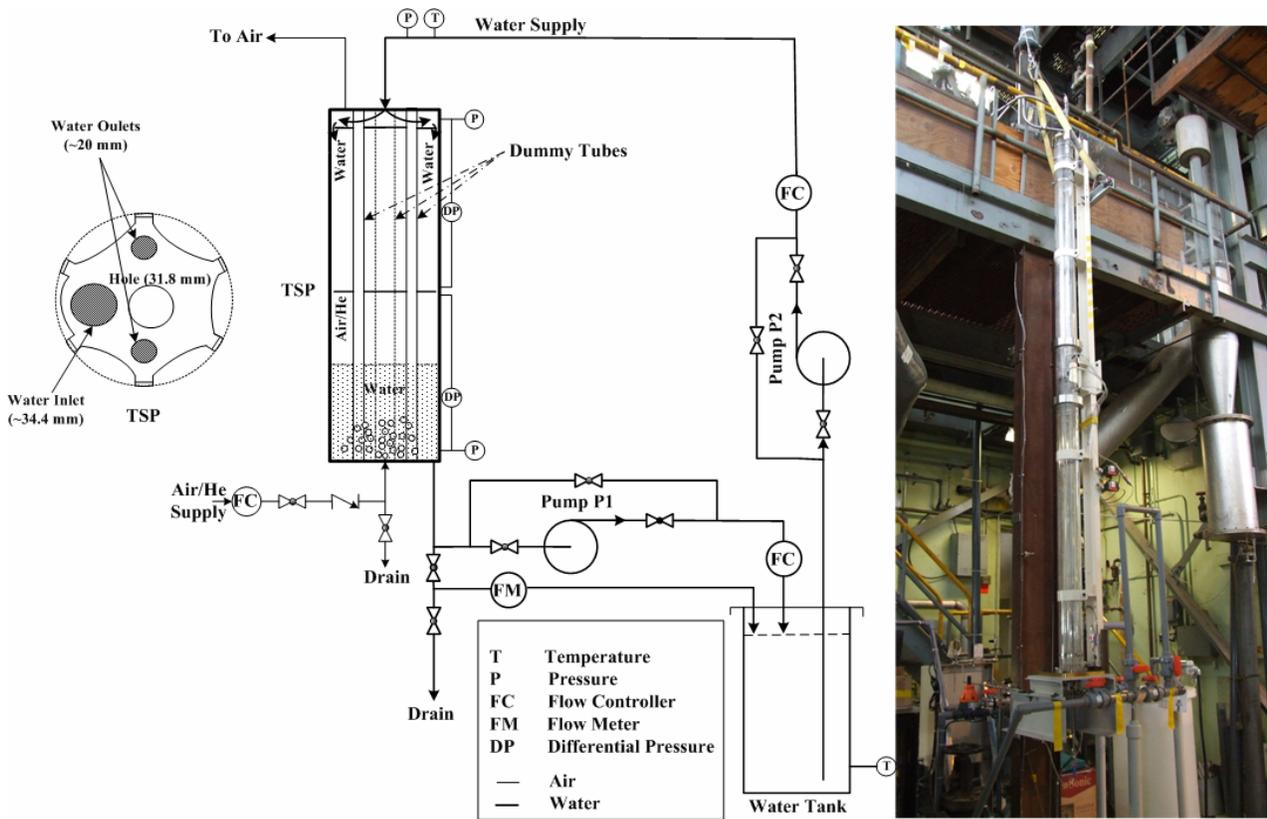
Figure 4: Schematic of the Experimental Set-up
