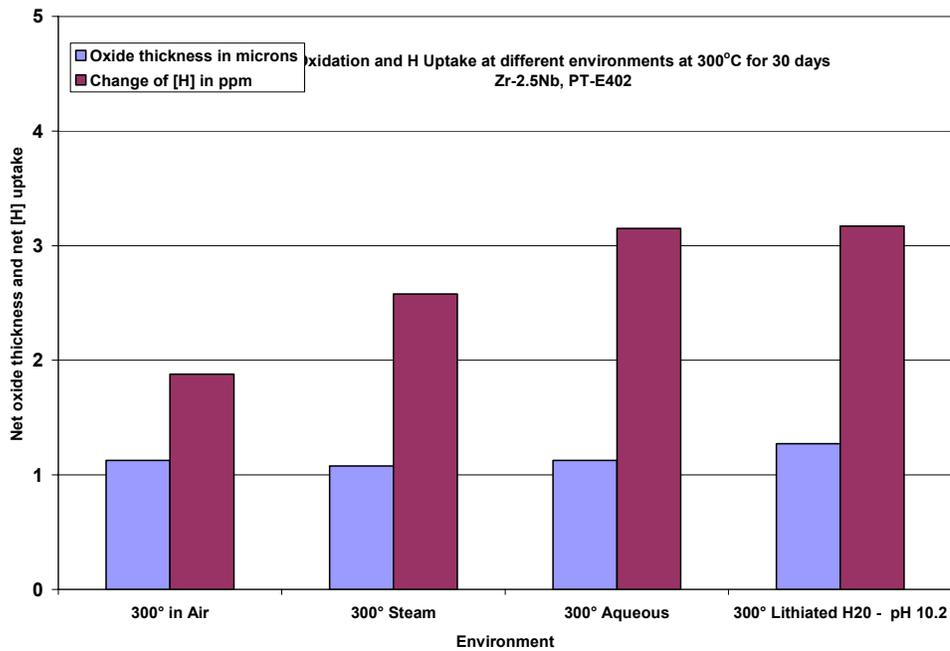
Figure 1b Oxidation and H pickup results for coupons from PT-E402 corroded in different environments for 30 days.
