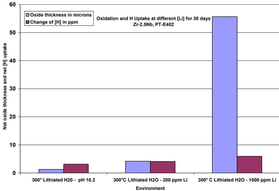
Figure 2b Oxidation and H pickup results for coupons from PT-E402 corroded in aqueous solution with increasing [Li] for 30 days.
