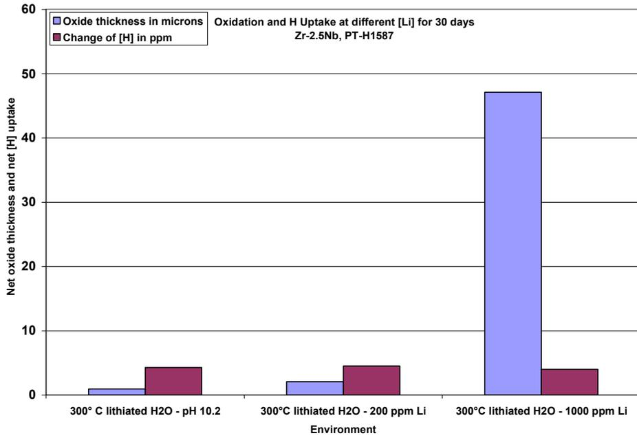
Figure 2a Oxidation and H pickup results for coupons from PT-H1587 corroded in aqueous solution with increasing [Li] for 30 days.
