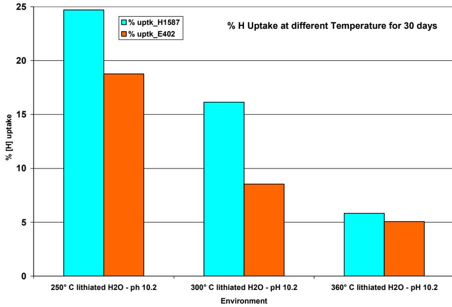
Figure 6 Percentage H uptake for coupons from both PTs (H1587 and E402) corroded in aqueous solution at increasing temperature for 30 days.
