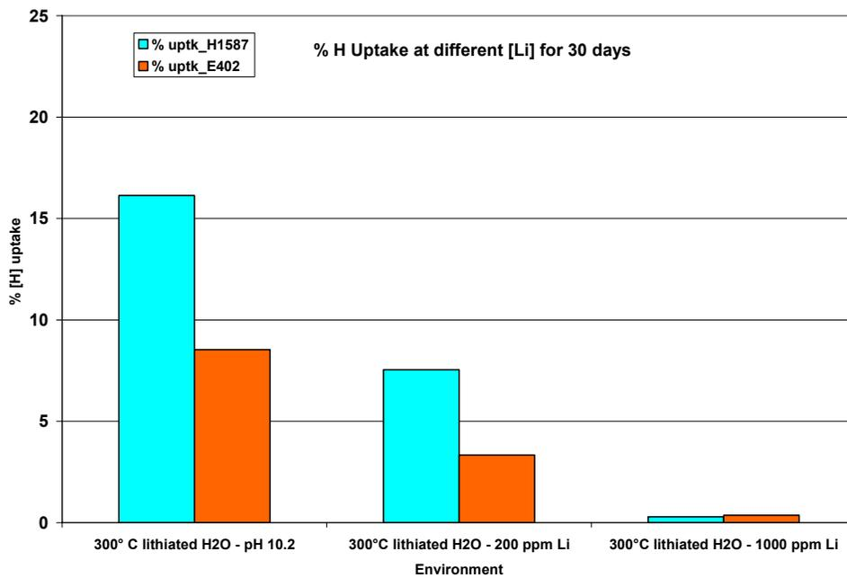
Figure 5 Percentage H uptake for coupons from both PTs (H1587 and E402) corroded in aqueous solution with increasing [Li] for 30 days.
