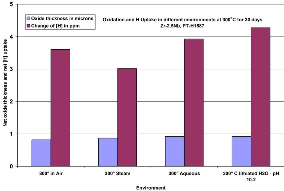
Figure 1a Oxidation and H pickup results for coupons from PT-H1587 corroded in different environments for 30 days.
