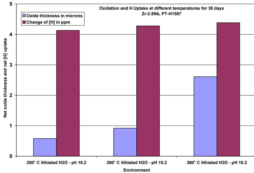
Figure 3a Oxidation and H pickup results for coupons from PT-H1587 corroded in aqueous solution at increasing temperature for 30 days.
