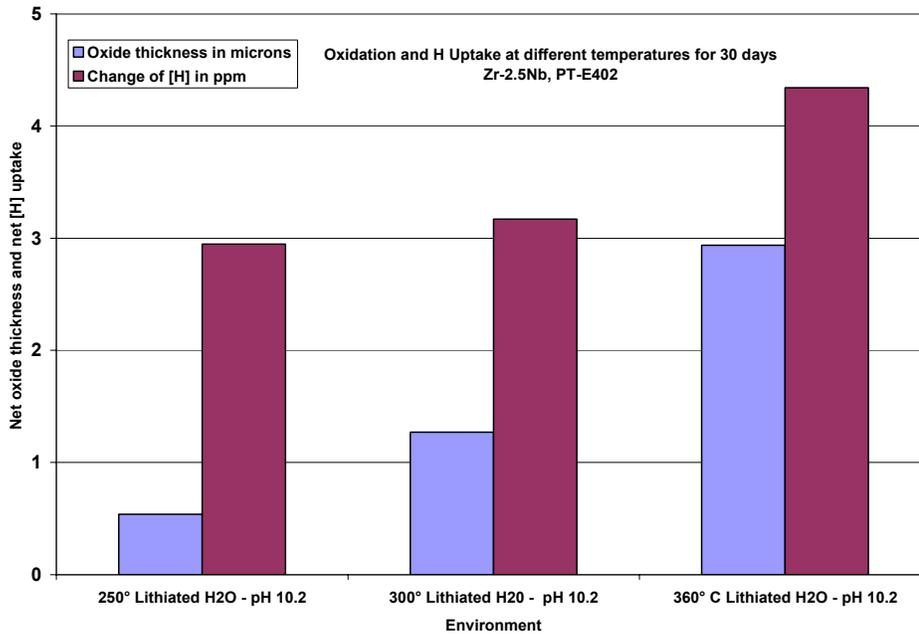
Figure 3b Oxidation and H pickup results for coupons from PT-E402 corroded in aqueous solution at increasing temperature for 30 days.
