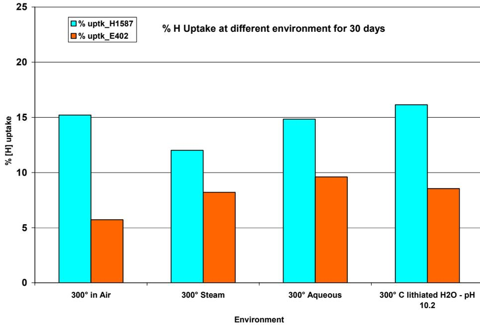
Figure 4 Percentage H uptake for coupons from both PTs (H1587 and E402) corroded under different environments for 30 days.
