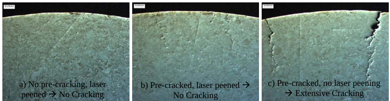
Figure 4: Alloy 600 U-bends immersed in sodium thiosulfate solution for two days. Figure a) laser peened then immersed in the thiosulfate solution. Figure b) immersed in the thiosulfate solution to generate cracks, laser peened, then re-immersed in the thiosulfate solution. Figure c) pre-cracked then re-immersed in the solution for comparison.
