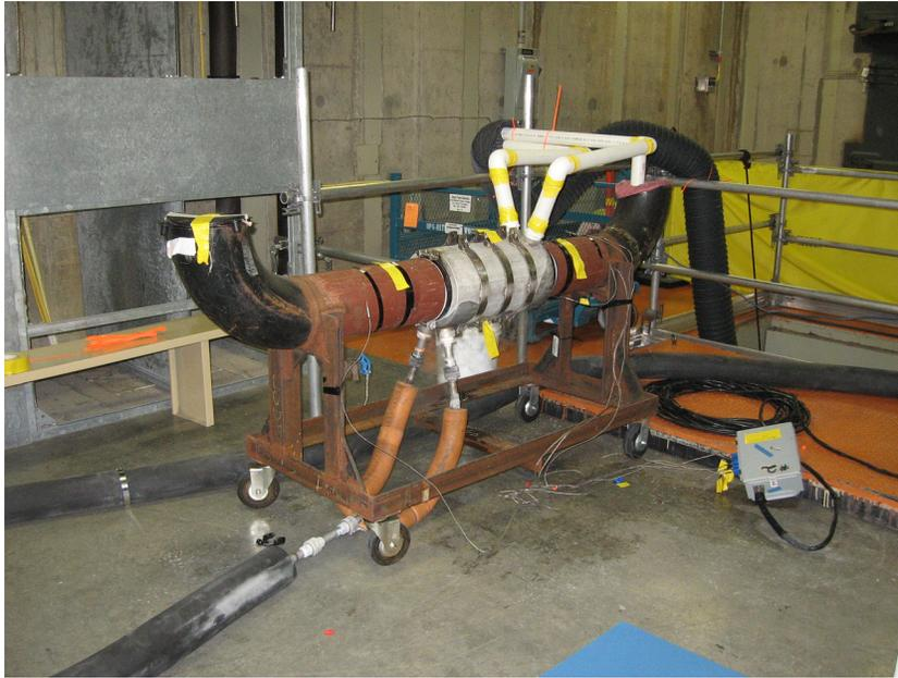
**Figure 9: Arrangement Ready to form Ice Plug on 8" Test Stand**
