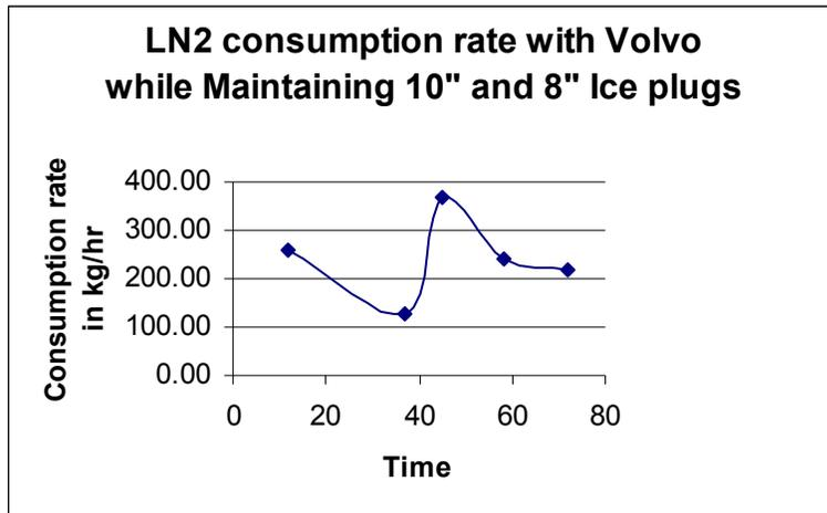
Figure 14: LN2 Consumption Rate to Maintain 10" and 8" Ice Plugs Using Volvo
