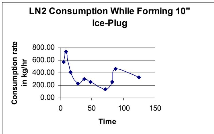
Figure 12: LN2 Consumption Rate While Forming 10" Ice plug in the 2<sup>nd</sup> Attempt
