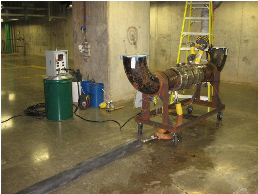
**Figure 8: Arrangement Ready to form Ice Plug on 10" Test Stand**
