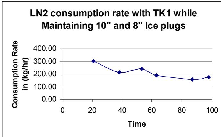
Figure 15: LN2 Consumption Rate to Maintain 10" and 8" Ice Plugs Using TK1
