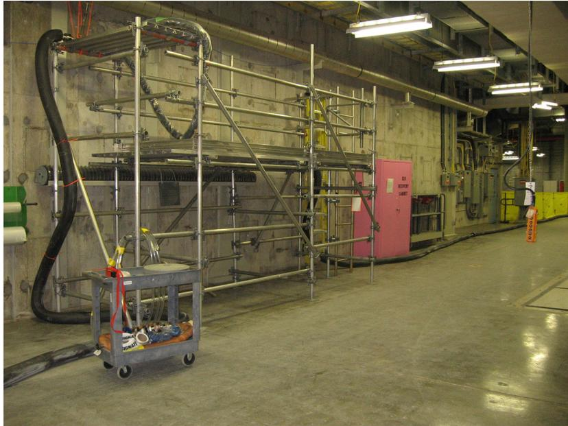
**Figure 5: Hoses Run Up the Scaffold to Simulate Containment Penetration**
