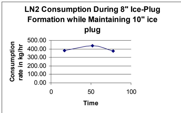
Figure 13: LN2 Consumption Rate While Forming 8" Ice plug and Maintaining 10" Ice Plug
