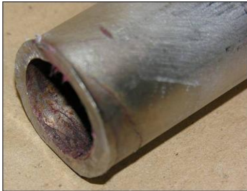
(a) 1" Ø pipe showing the cracking
