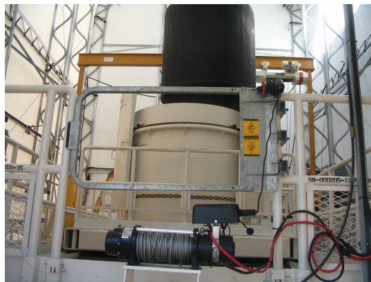
Figure 3: Resin Liner being Lowered into Overpack Pre-Staged in Process Shield
