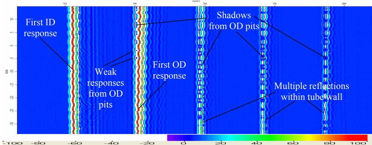
Figure 9. PE NB axial B-scan of pressure tube with angle row of OD pits 0.7mm wide and 0.7mm deep. Axially positioned probe with attached  $45^\circ$  conical mirror. Probe: center frequency  $f=10\text{MHz}$ , focal length  $FL=100\text{mm}$ , diameter  $D=9.5\text{mm}$ , water-path  $WP=45\text{mm}$ .
