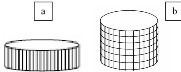
Figure 1. Schematics of 1D circular cylindrical array (a) and 2D cylindrical matrix array (b).
