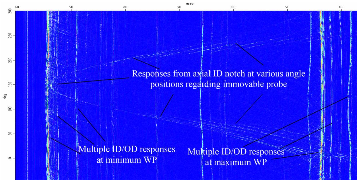
Figure 11. PE 360° circumferential B-scan of pressure tube with one axial rectangular ID notch 2.5mm wide and 0.5mm deep. Axially positioned probe with attached 45° conical mirror was located eccentrically in relation to the tube. Probe:  $f=10\text{MHz}$ ,  $FL=100\text{mm}$ ,  $D=9.5\text{mm}$ , minimum water-path between tube and mirror  $WP=20\text{mm}$  (signal arrives at  $45\mu\text{s}$ ), maximum  $WP=60\text{mm}$  (signal arrives at  $97\mu\text{s}$ ). Color scale is shown in Fig. 9.
