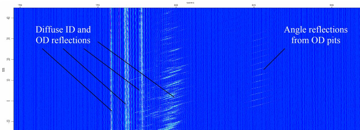
Figure 10. PE angle shear wave axial B-scan of pressure tube with angle row of OD pits 0.7mm wide and 0.7mm deep. Axially positioned probe with attached  $35^\circ$  conical mirror. Probe:  $f=10\text{MHz}$ ,  $FL=100\text{mm}$ ,  $D=9.5\text{mm}$ ,  $WP=45\text{mm}$ . Color scale is shown in Fig. 9.
