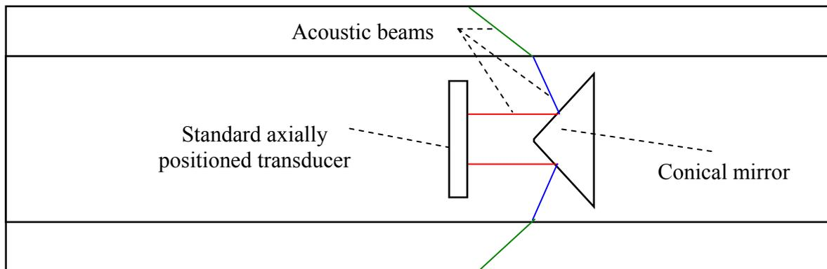
Figure 5. Schematics of angle shear wave probe, containing axially positioned standard transducer with attached  $35^{\circ}$  conical mirror for circumferential flaws detection.
