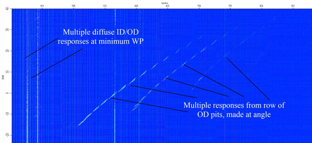
Figure 13. PE axial B-scan of tube with angle row of OD pits 0.7mm wide and 0.7mm deep. Axially positioned probe with attached  $35^{\circ}$  conical mirror was located eccentrically in relation to the tube. Probe:  $f=10\text{MHz}$ ,  $FL=100\text{mm}$ ,  $D=9.5\text{mm}$ , minimum  $WP=18\text{mm}$  (signal arrives at  $40\mu\text{s}$ ), maximum  $WP=64\text{mm}$  (signal arrives at  $111\mu\text{s}$ ). Color scale is shown in Fig. 9.
