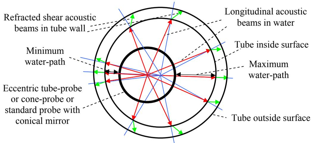
Figure 7. Schematic of top view of NB tube-probe or angle shear wave cone-probe positioned eccentrically in relation to the tube (or eccentrically positioned and axially oriented standard probe with attached conical mirror) for axial flaw detection.
