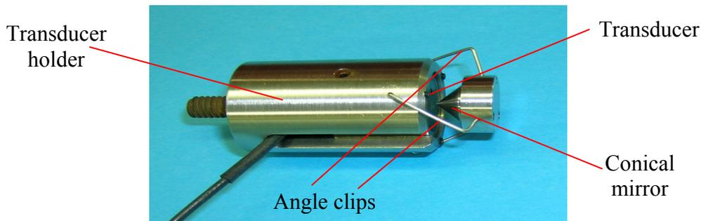
Figure 8. Picture of axially positioned standard probe with attached conical mirror.
