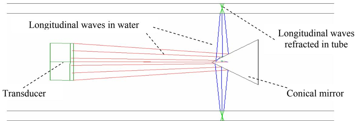
Figure 4. Schematics of NB probe, containing axially positioned standard focused transducer with attached  $45^{\circ}$  conical mirror.
