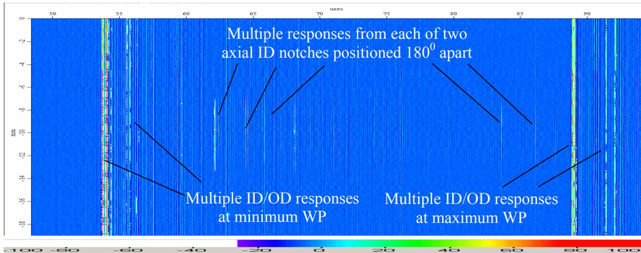
Figure 14. PE axial B-scan of PT with two axial ID notches 0.15mm wide and 0.15 and 0.076mm deep positioned 180° apart. Axially positioned probe with attached 45° conical mirror was located eccentrically in relation to the tube. Probe: f=10MHz, FL=100mm, D=9.5mm, minimum WP=30mm (signal arrives at 54μs), maximum WP=50mm (signal arrives at 89μs).
