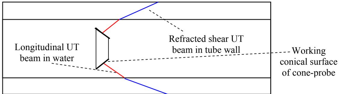
Figure 3. Schematics of angle shear wave cone-probe for circumferential flaw detection.
