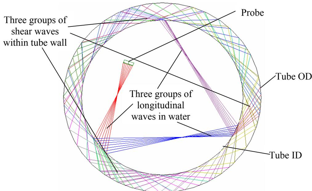
Figure 15. Ray-tracing simulation of shear wave multi-skip technique.
