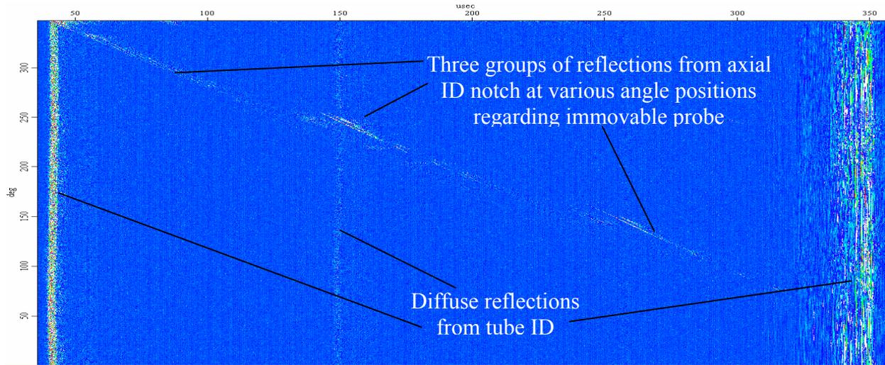
Figure 16. Circumferential PE B-scan of axial rectangular ID notch 0.5mm deep and 2.5mm wide. Probe: D=9.5mm, f=10MHz, FL=40mm, WP=22mm, offset 13mm, incident angle  $36^{\circ}$ . Color scale is given in Fig. 9.
