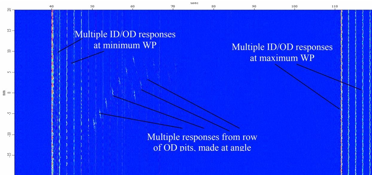
Figure 12. PE axial B-scan of tube with angle row of OD pits 0.7mm wide and 0.7mm deep. Axially positioned probe with attached  $45^{\circ}$  conical mirror was located eccentrically in relation to the tube. Probe:  $f=10\text{MHz}$ ,  $FL=100\text{mm}$ ,  $D=9.5\text{mm}$ , minimum  $WP=18\text{mm}$  (signal arrives at  $40\mu\text{s}$ ), maximum  $WP=64\text{mm}$  (signal arrives at  $111\mu\text{s}$ ). Color scale is shown in Fig. 9.
