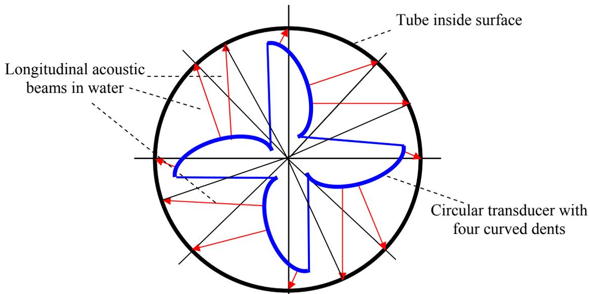
Figure 6. Schematic of angle shear wave circular transducer with four curved dents for axial flaws detection; UT beams impinge on the tube surface everywhere at the same incident angle.
