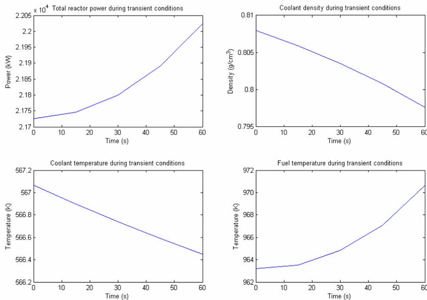
Figure 10. Transient simulations for outlet pressure decrease.
