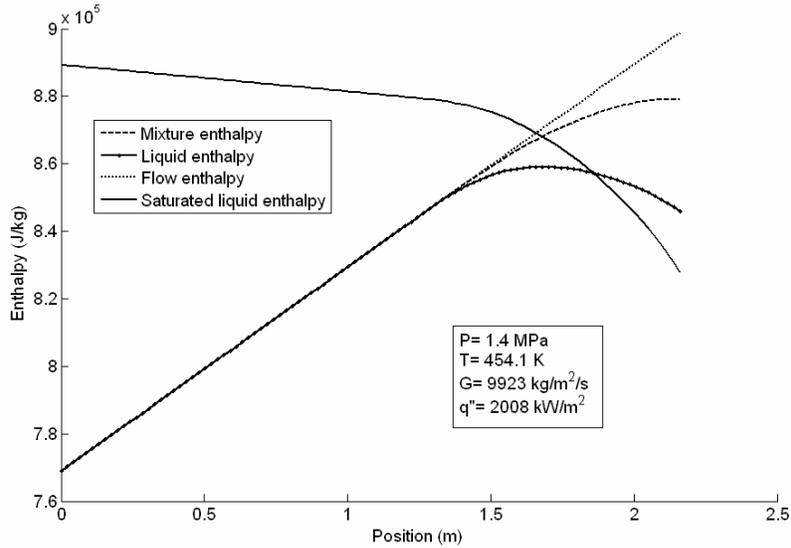
Figure 5: Flow and mixture enthalpy.
