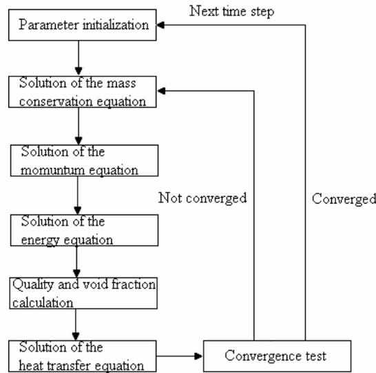
Figure 7. ARTHUR's thermal calculation algorithm.
