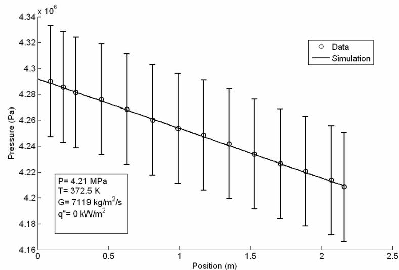
Figure 1. Comparison of simulated vs. measured pressure drop under single-phase flow conditions [6].
