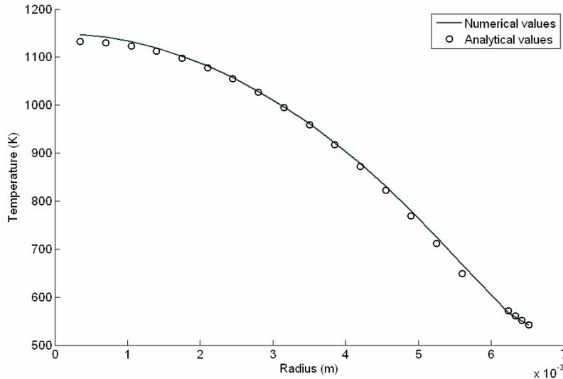
Figure 6. Radial temperature distribution in a typical fuel pin.
