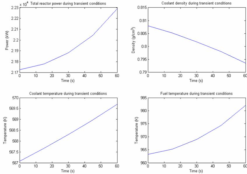
Figure 11. Transient simulations for a decrease of the inlet subcooling.
