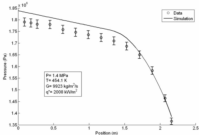
Figure 3: Axial pressure drop profile vs. data given in [6].
