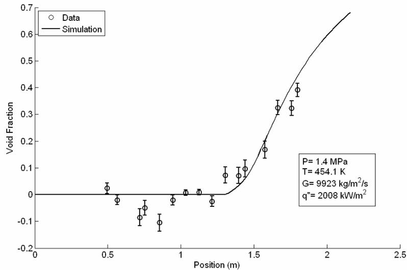
Figure 2: Axial void fraction distributions vs. data given in [6].
