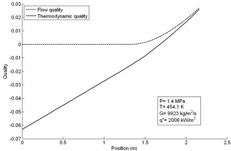
Figure 4: Calculated thermodynamic and flow qualities.
