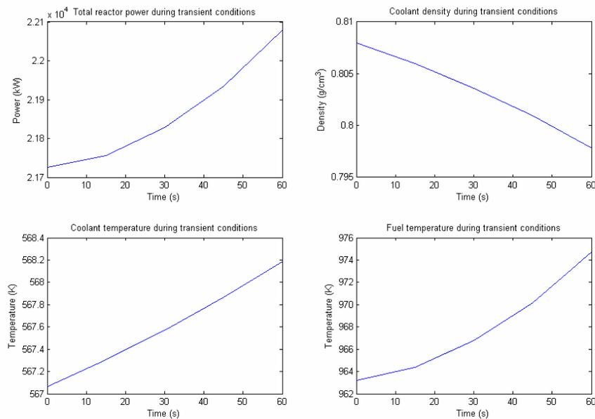
Figure 9. Transient simulations for a decrease of the inlet mass flow rate.
