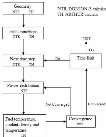
Figure 8. Coupled neutronic/thermohydraulic calculation algorithm.
