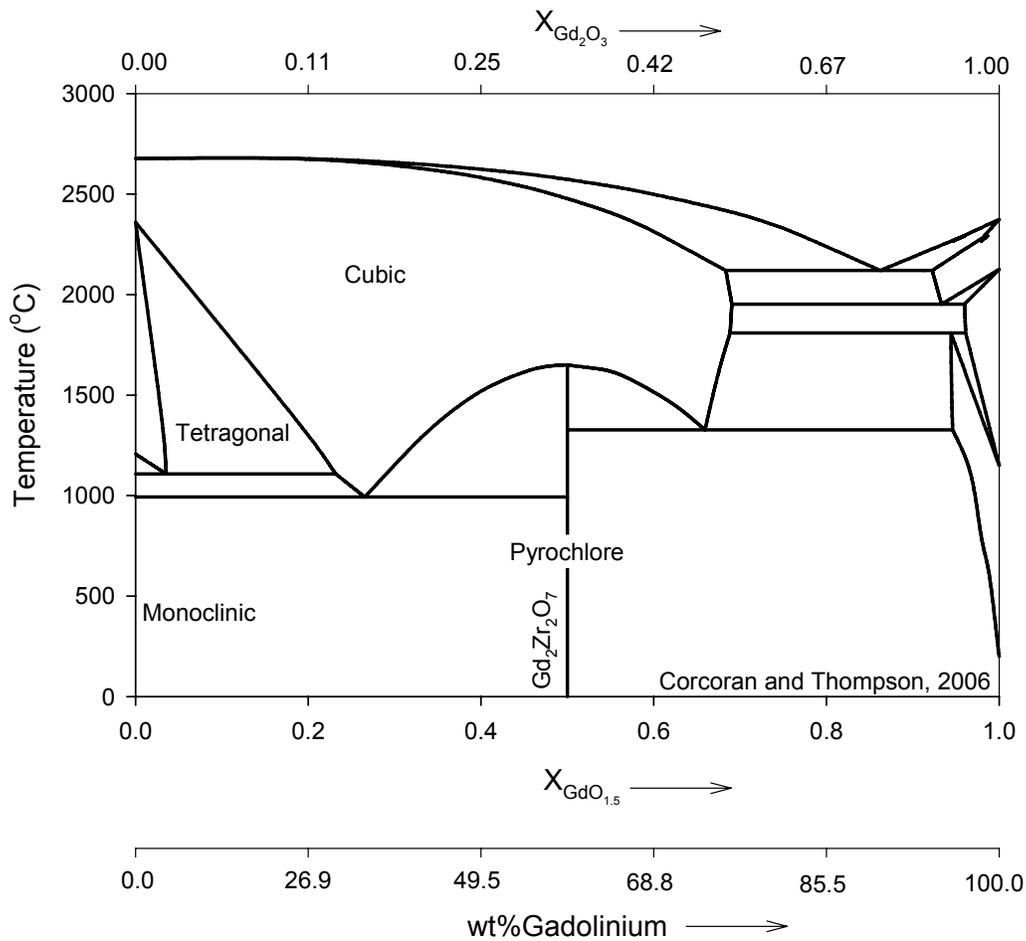
**Figure 1: ZrO<sub>2</sub>-Gd<sub>2</sub>O<sub>3</sub> Binary Phase Diagram**
