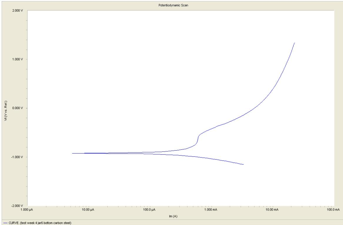
Figure 4 Potentiodynamic scan for unsealed carbon steel coupon, no chloride, located at the bottom of the jar, November 14, 2006.
