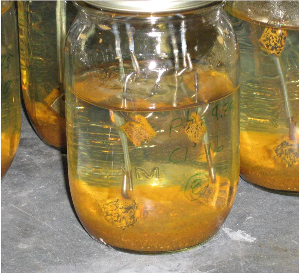
Figure 1 Carbon steel coupons in Mason jar after 91 days
