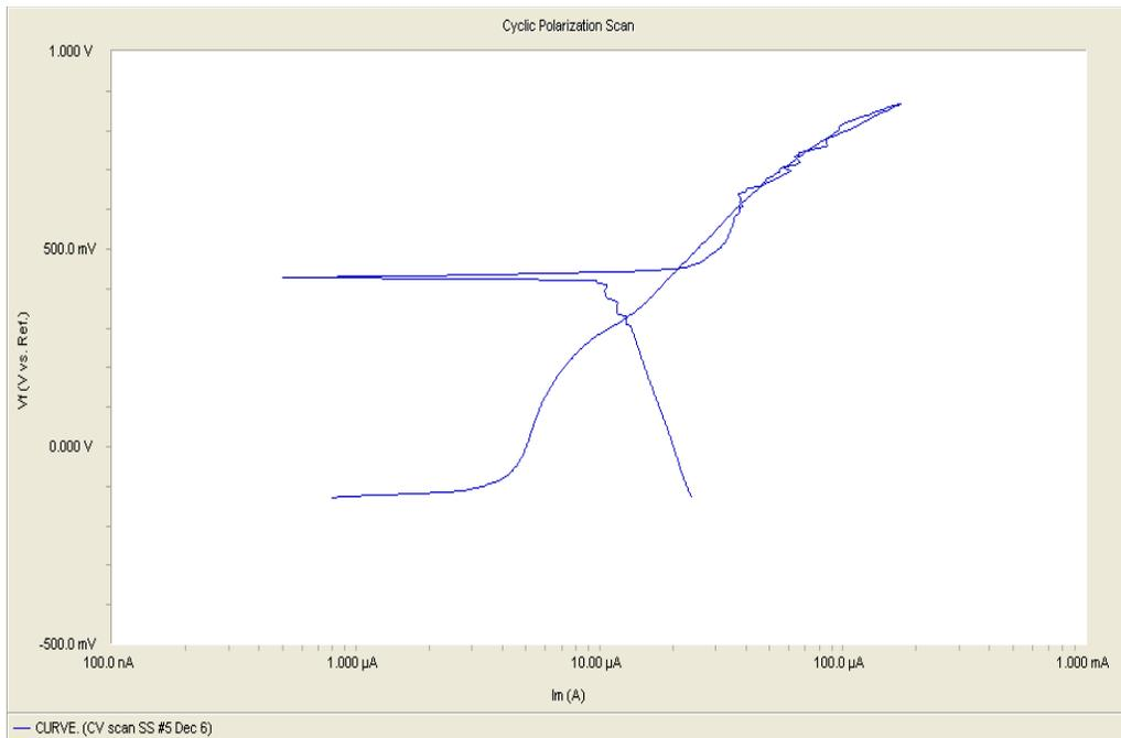
Figure 6 Pitting potential for stainless steel coupon with chloride, located at the top of a sealed jar, December 5, 2006. Pitting potential is ambiguous.
