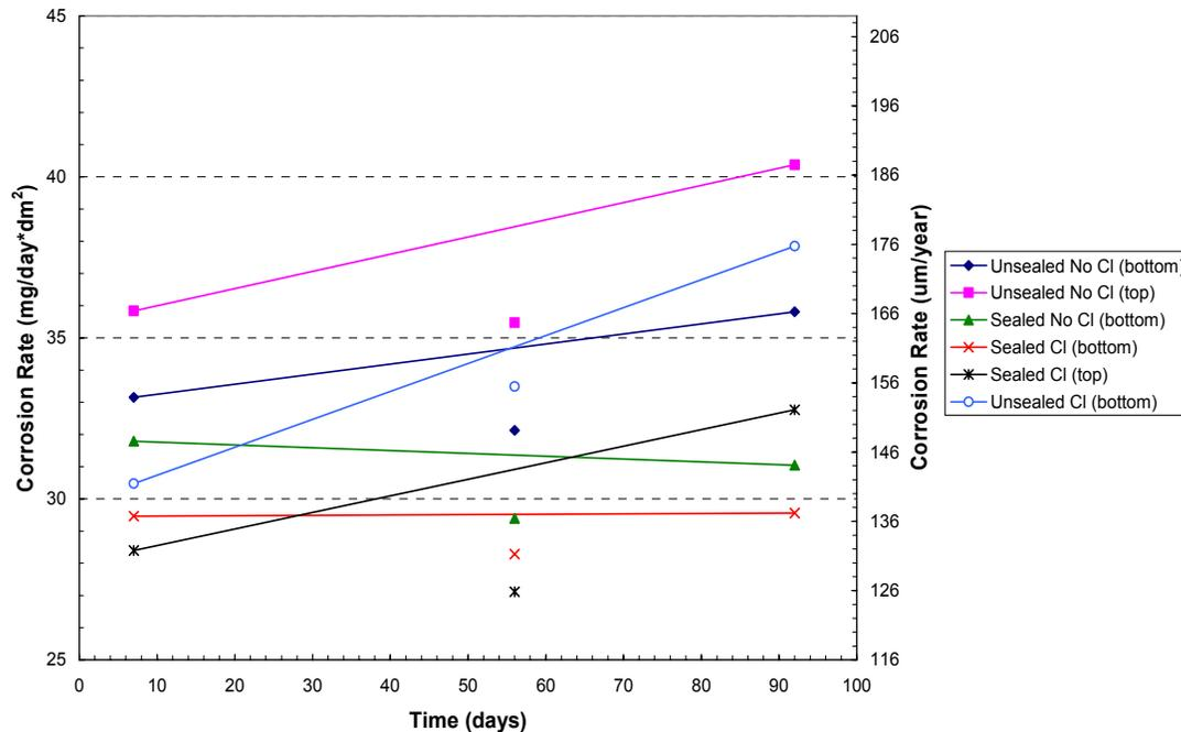
Figure 3 Corrosion rates of all carbon steel coupons
