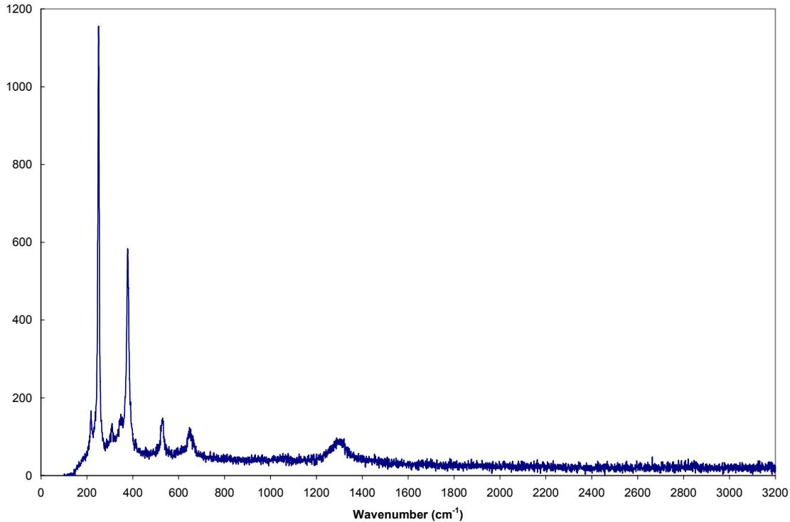
Figure 7 Raman spectrum of Mason jar corrosion product
