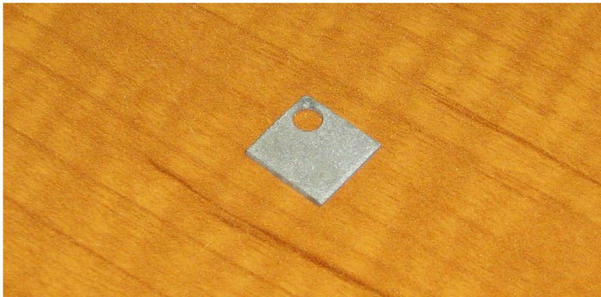
Figure 2 Carbon steel sample after descaling
