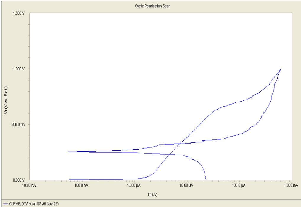
Figure 5 Pitting potential for stainless steel coupon with chloride, located at the top of a sealed jar, November 29, 2006. Pitting potential is 630mV.
