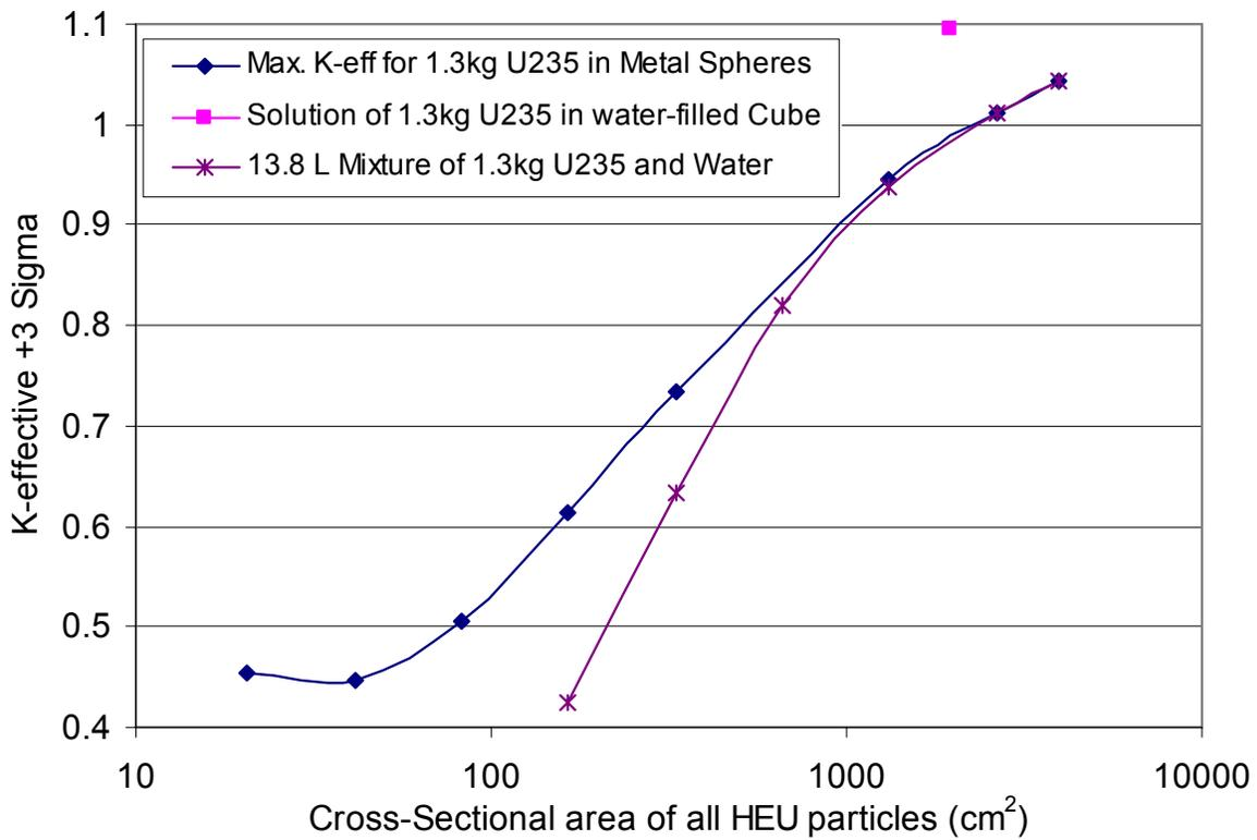
Figure 3 :  $K$ -effective +  $3\sigma$  for  $^{235}\text{U}$  as a function of macroscopic cross-sectional area of HEU particles in water-filled cube
