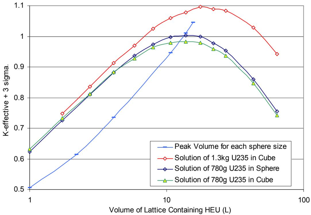
Figure 2 :  $K$ -effective +  $3\sigma$  for up to 1.3kg  $^{235}\text{U}$  as a function of volume
