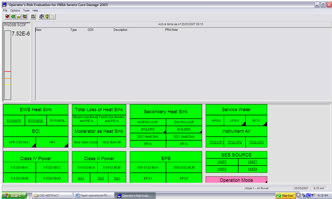
Figure 1: Screenshot of the Operator Screen of the Pickering NGS B At-Power Risk Monitor (EOOS) – Zero Maintenance Condition
