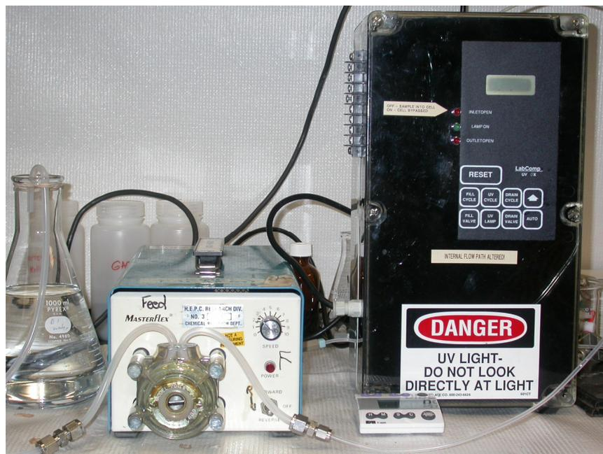
Figure 2 UV Oxidation Set-up
