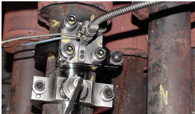
Figure 3 Installed HEP (top) and FOLTM (bottom) on PHT feeder
