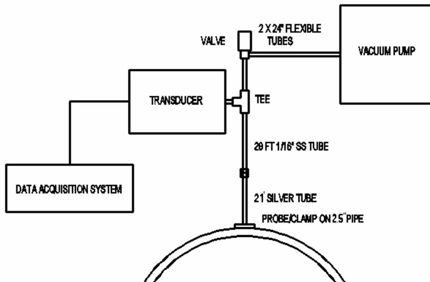
Figure 2 Schematic of HEP components
