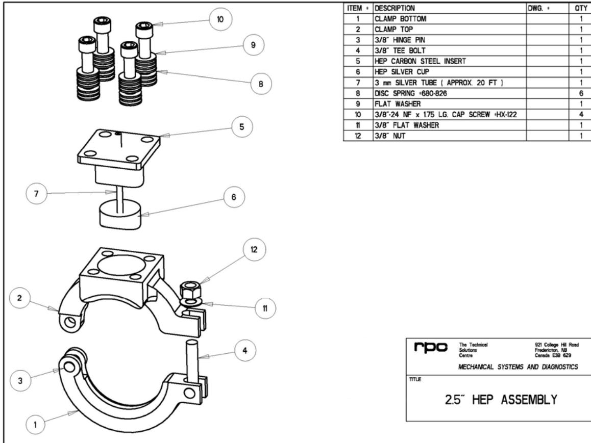
Figure 1 HEP annulus and clamping apparatus
