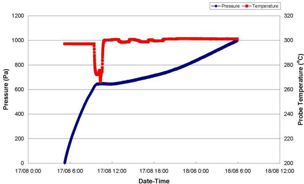
Figure 6 HEP pressure increase during fuelling
