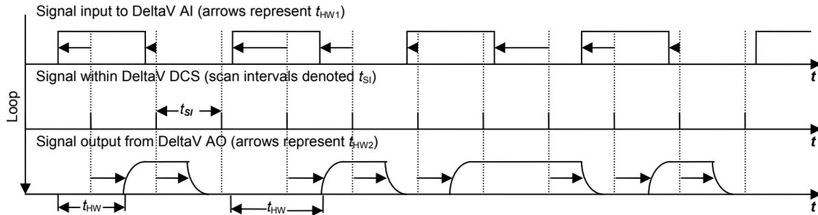
Figure 2 Timing diagram of the DeltaV DCS using hardwires
