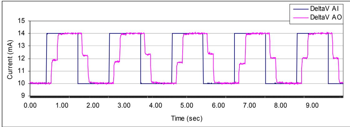
Figure 3 Test results when the scan rate is set to be 200ms
