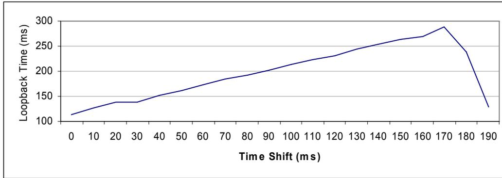
Figure 4 Average loop-back time relative to the time shifts at the scan rate of 200ms
