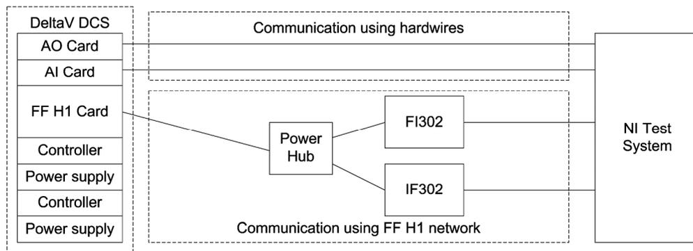
Figure 1 Framework of test-bench
