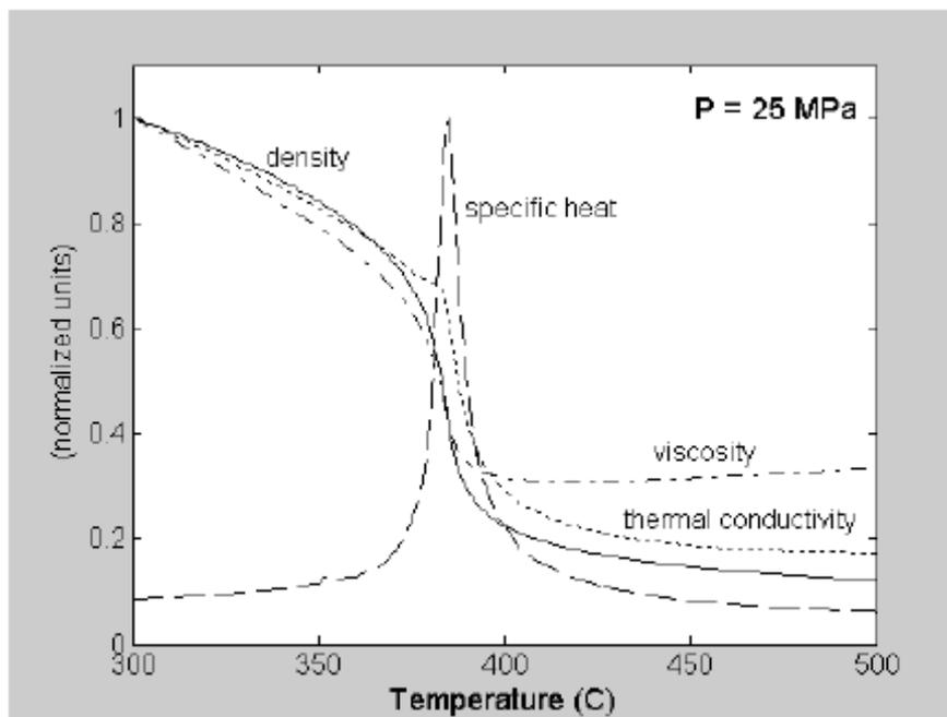
Figure 4: Thermal variation of physical properties of water, showing clearly the specific heat peak at the critical point. Density, viscosity and thermal conductivity are seen to decline significantly with temperature. A major consequence of the higher specific heat of supercritical water is that a far more efficient heat transfer can take place through the coolant, reducing the amount of mass flow required in the loop.
