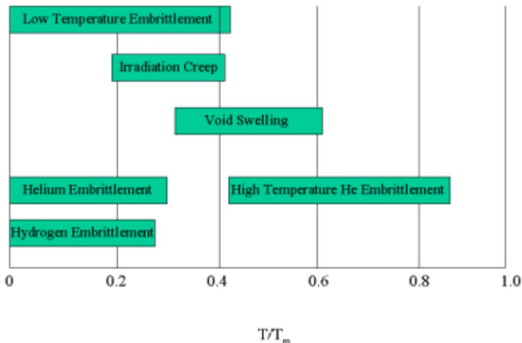
Figure 6: A diagram sketching out the different damage regimes applicable to alloys used in reactor materials, as a function of the homologous temperature. (Homologous temperature is the temperature in fractions of melting temperature.) From [12].
