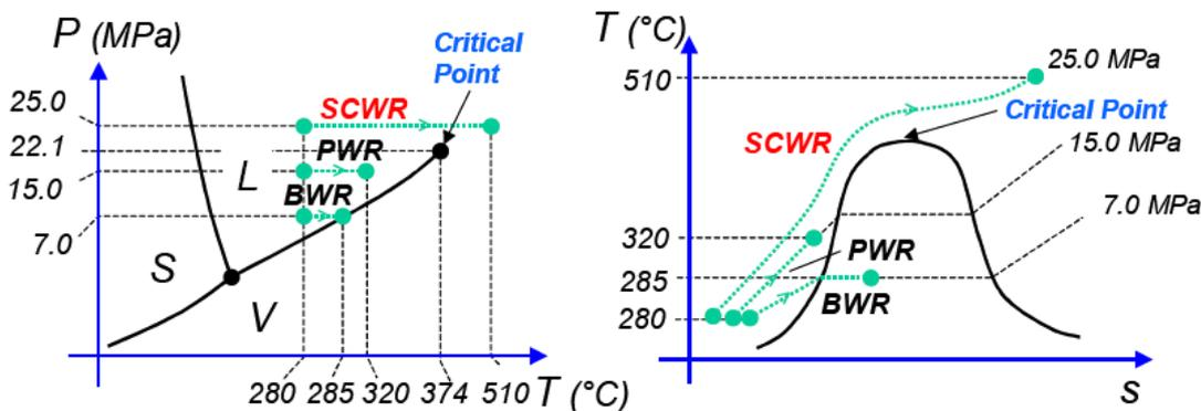
Figure 1: *Left*: Phase diagram of water, showing the critical point and the relative operating regimes of the Supercritical Water Reactor (SCWR), the Pressurized Water Reactor (PWR), and the Boiling Water Reactor (BWR). The reference temperature shown is that of the US SCWR variant, while the CANDU-SCWR outlet temperature is higher, at 650 C. *Right*: Temperature-Entropy diagram of water, showing the greater heat transfer possible above the supercritical point. From [7].
