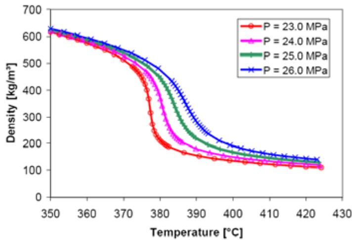
Figure 3: Density changes in supercritical water as a function of pressure and temperature. From [11]
