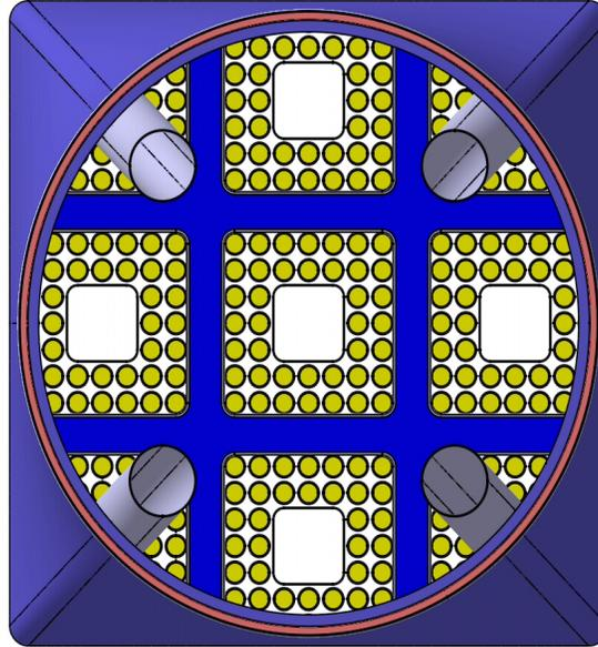
Figure 1: View through the head piece onto the HPLWR fuel assembly cluster [7].
