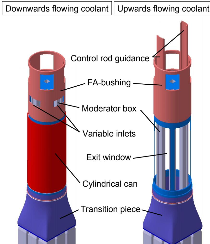
Fig. 6 Modified head piece to enable upward and downward flow
