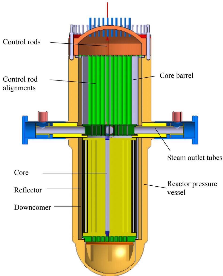
Figure 5: Reactor pressure vessel design [14].
