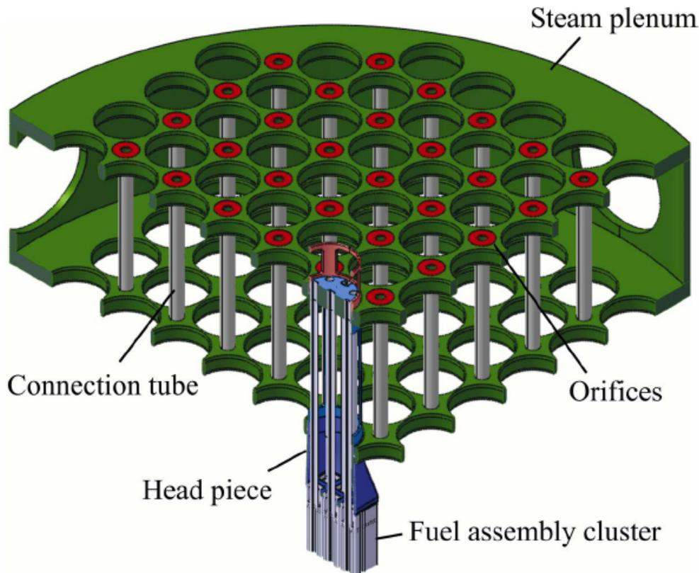
Figure 3: Steam plenum and head piece of a single pass core design [7].
