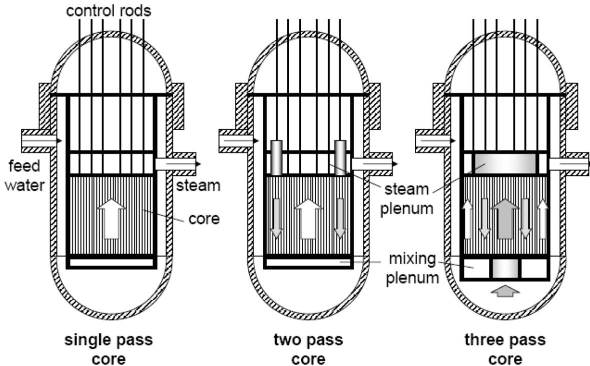
Figure 2: Core design concepts with multiple heat-up steps
