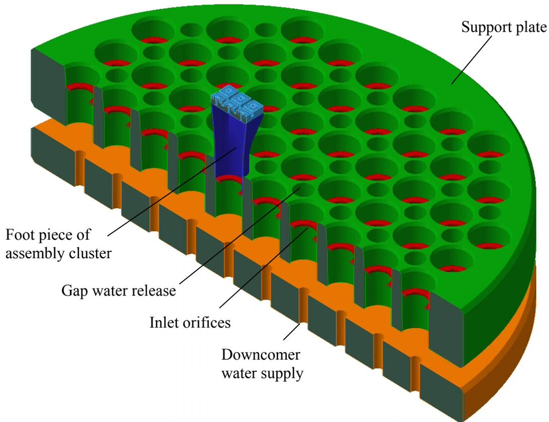
Figure 4: Foot piece and support plate with orifices of a single pass core design [18].
