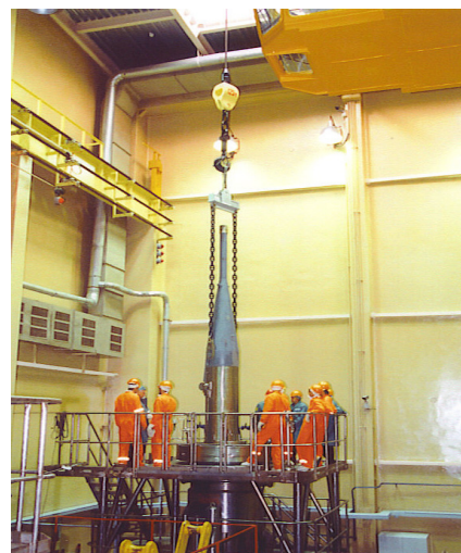
B - Loading of transfer flask with SNF assembly into SNF cask
