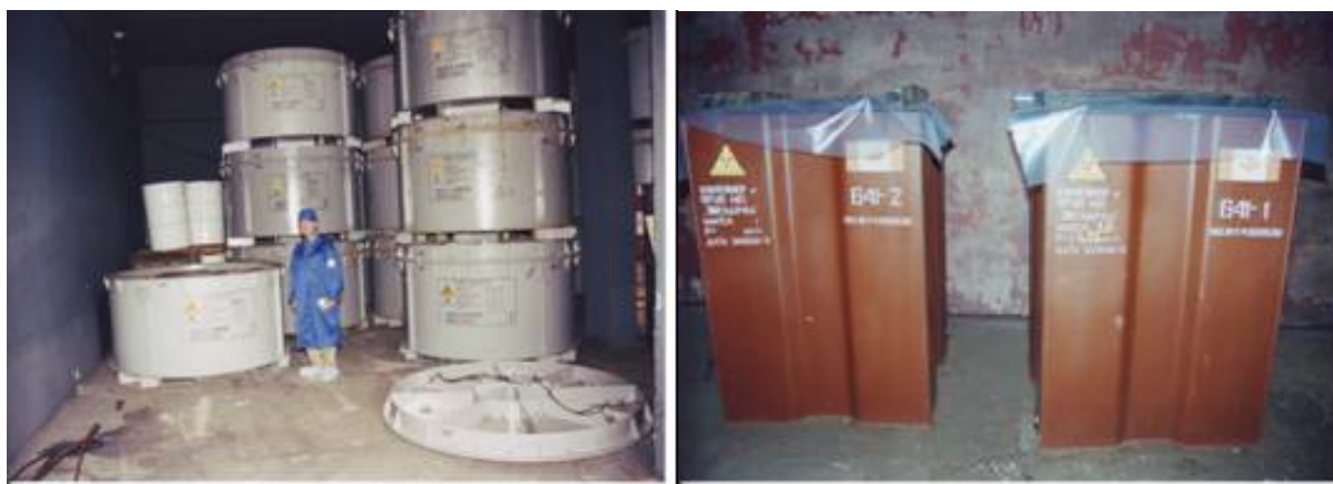
Figure 6: Solid Radioactive Waste Management - Intermediate Level Waste containers (left) and Low Level Waste containers.
