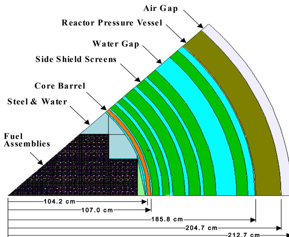
Figure 6 Simplified Reactor Structure of SMART for the GEOSHIELD Modelling
