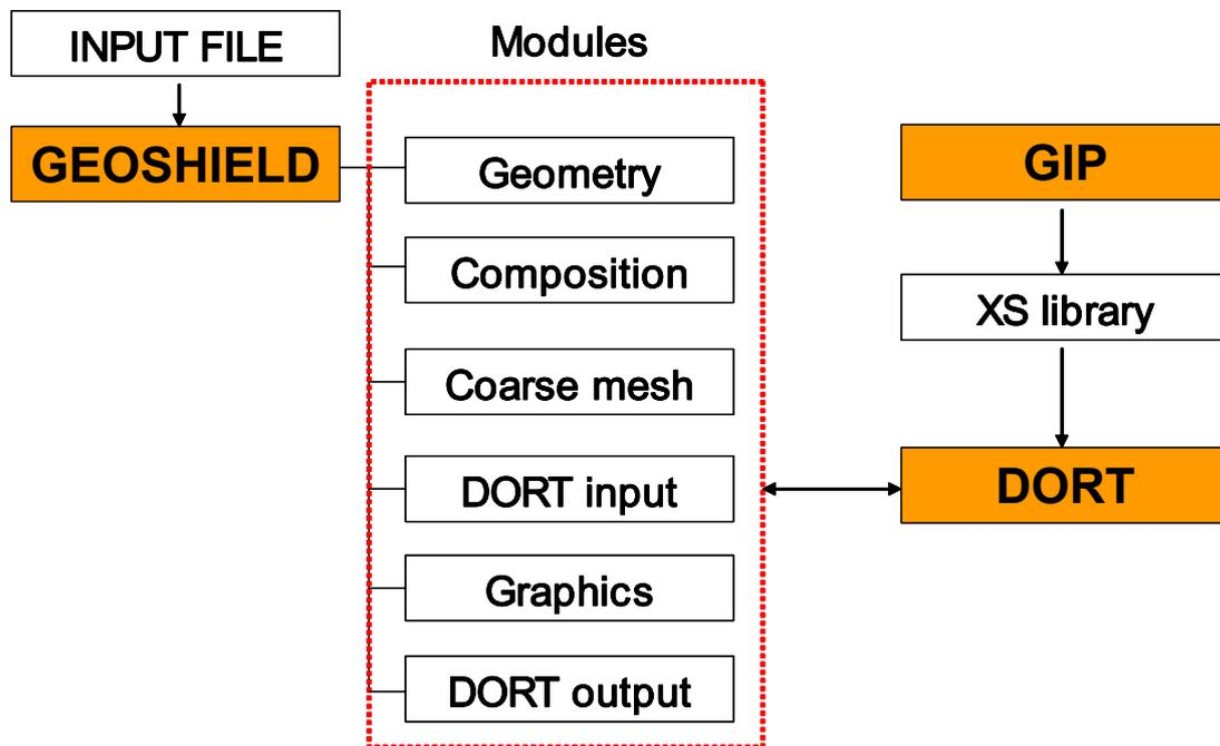
Figure 2 Flow chart of the GEOSHIELD calculation
