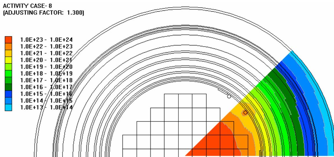
Figure 10 Fast neutron fluence distribution using GEOSHIELD code system [neutrons/cm<sup>2</sup>]
