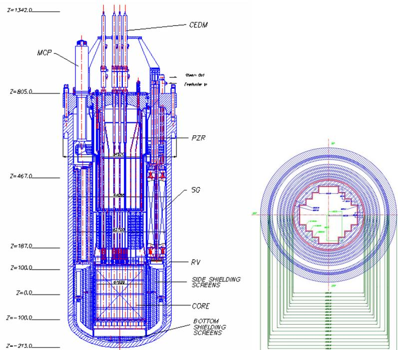
Figure 1 SMART Reactor Assembly and cross-sectional view
