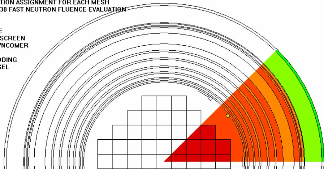
Figure 9 Composition assignment for each mesh of the DORT model using GEOSHIELD
