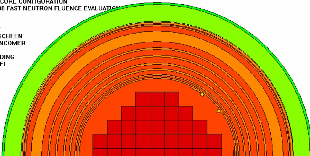
Figure 7 Original reactor configuration for the DORT model using GEOSHIELD
