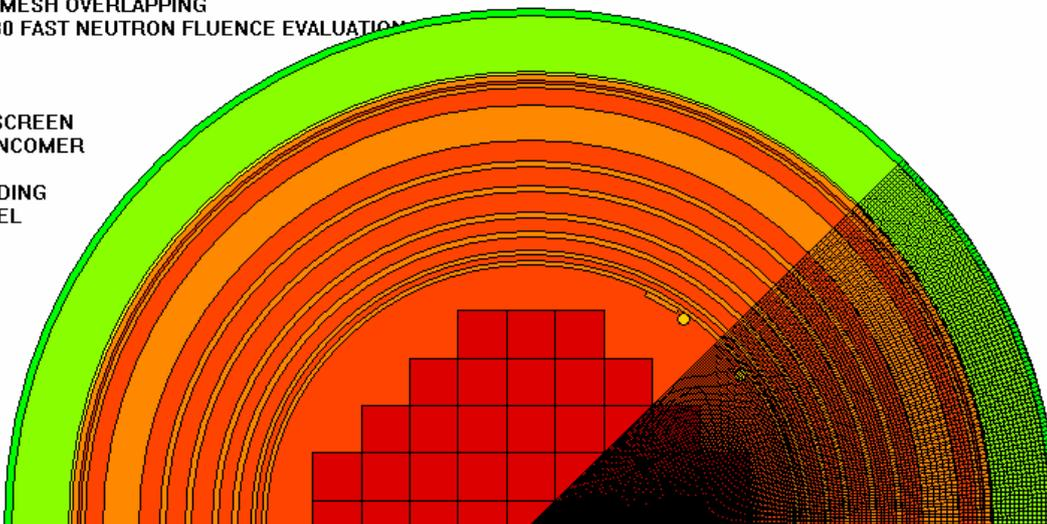
Figure 8 Regular mesh overlapping for the DORT model using GEOSHIELD
