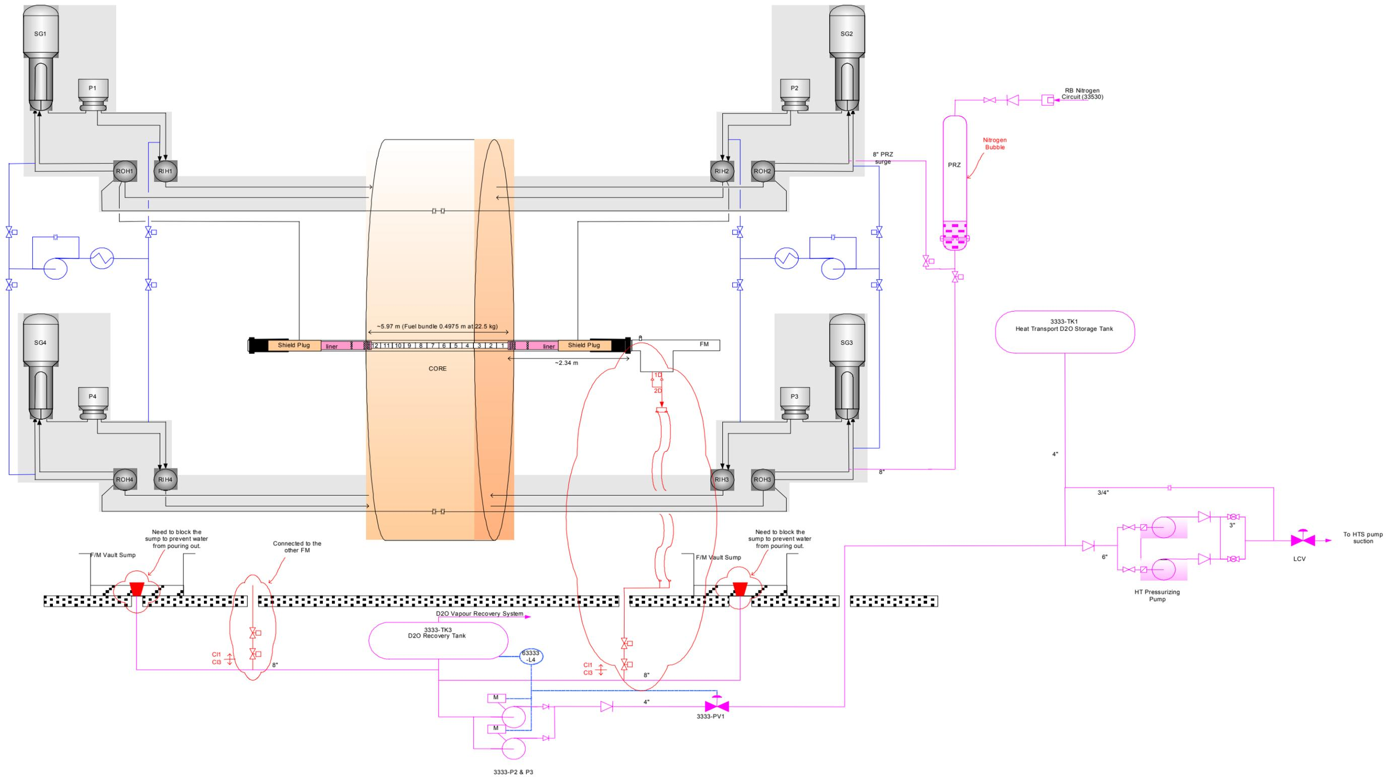
Figure 1: Through Flow Defuelling Proposed Arrangement
