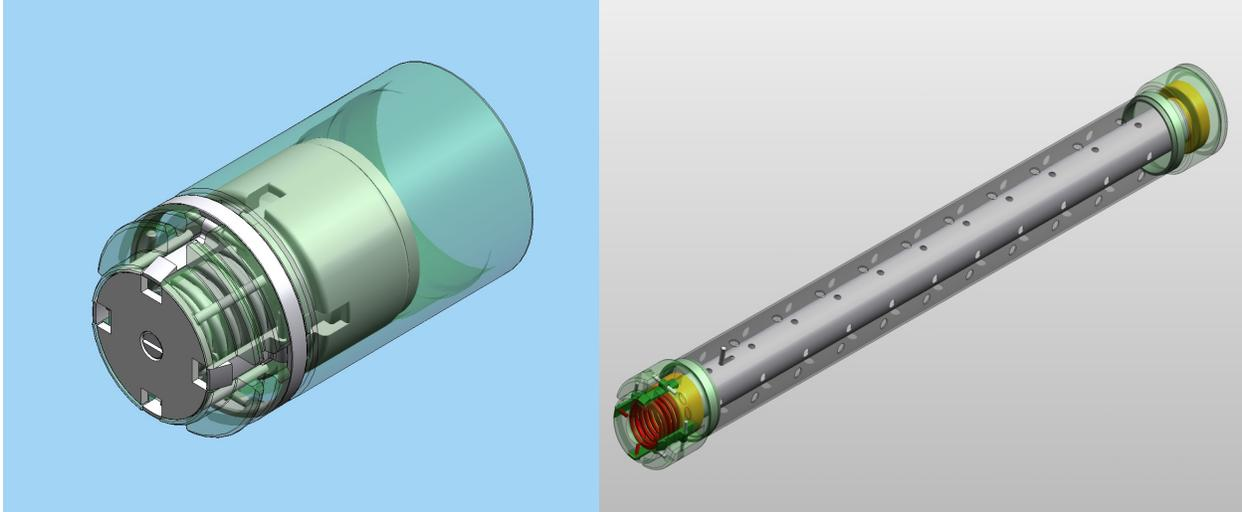
Figure 2: Ram Grapple Adaptor and Fuel Grapple Extension
