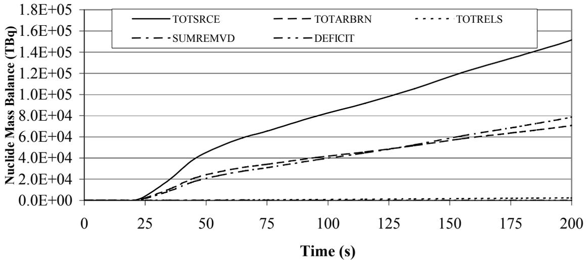
**Figure 8: Mass balance of nuclides among the quantities: a) source (TOTSRC), b) airborne in the containment atmosphere (TOTARBRN), c) escaped to the outside atmosphere (TOTRELS), d) removed from the containment atmosphere (SUMREMVD), and e) deficit.**
