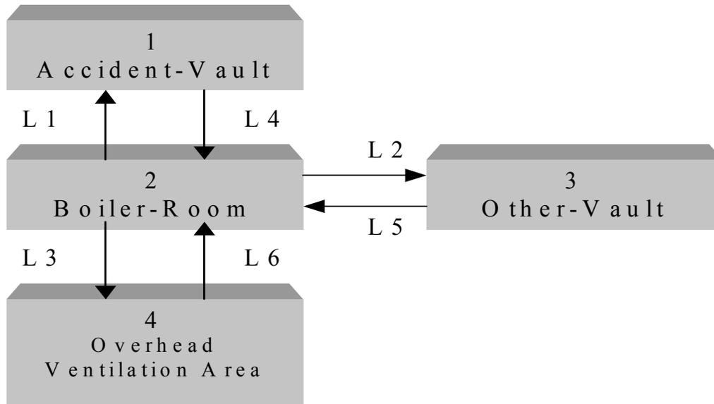
Figure 2: Containment geometry model represented by a network of rooms (nodes) interconnected by flow paths (links)
