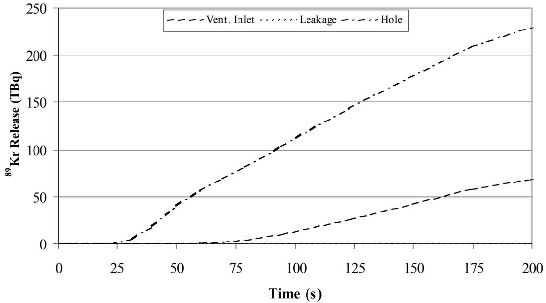
**Figure 7: Cumulative quantity of  $^{89}\text{Kr}$  released to the outside atmosphere through different release paths**
