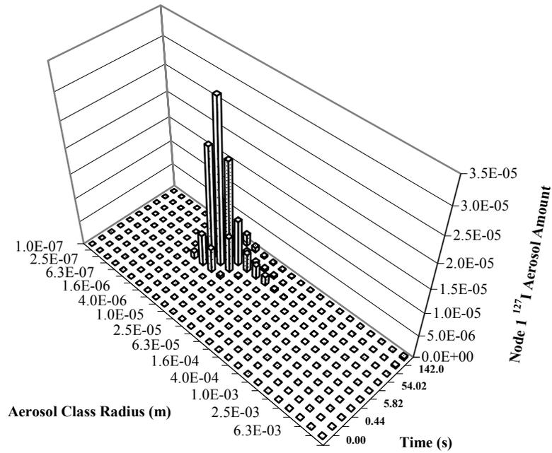
**Figure 4:  $^{127}\text{I}$  present in aerosols of different class sizes and its change with time in Accident-Vault (Node #1)**
