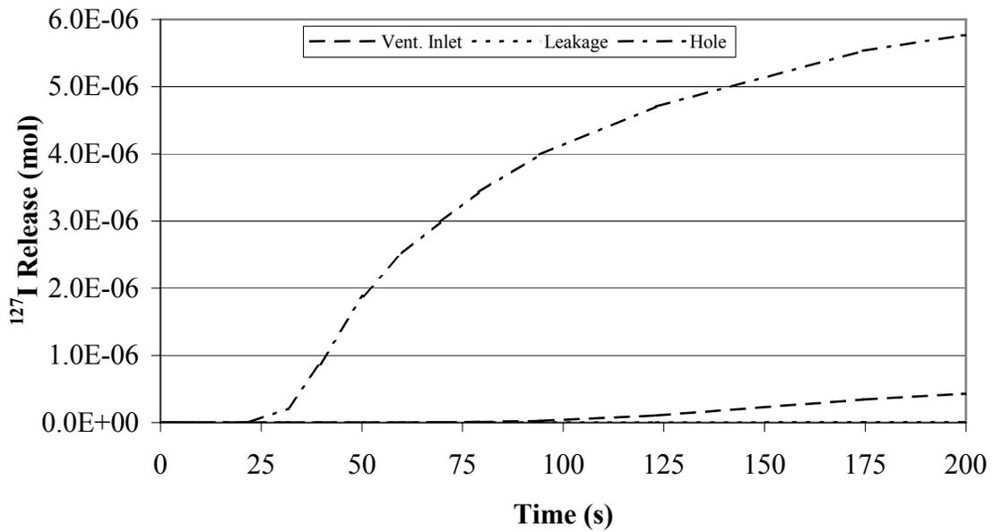
**Figure 6: Cumulative quantity of <sup>127</sup>I released to the outside atmosphere through different release paths**
