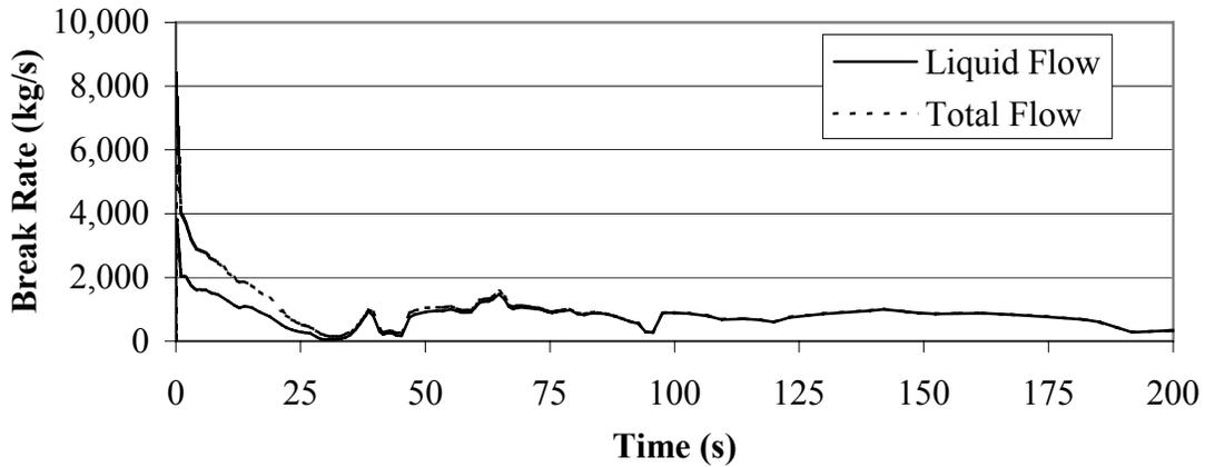
**Figure 3: Break flow transients showing the total flow consisting of both water and steam and the water portion of the total flow**
