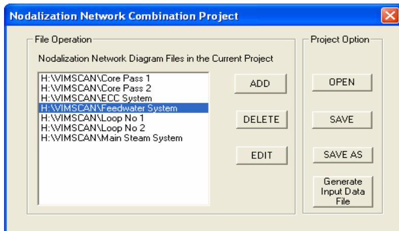
Figure 4 Workspace window for combining nodalization networks
