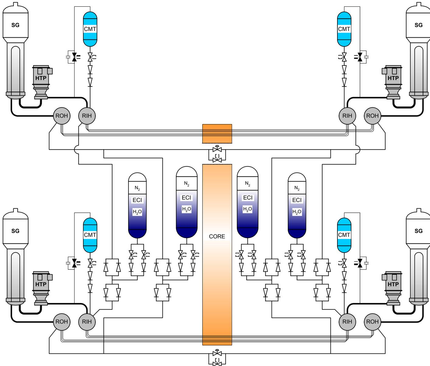
Figure 1 ACR-1000 Emergency Coolant Injection System
