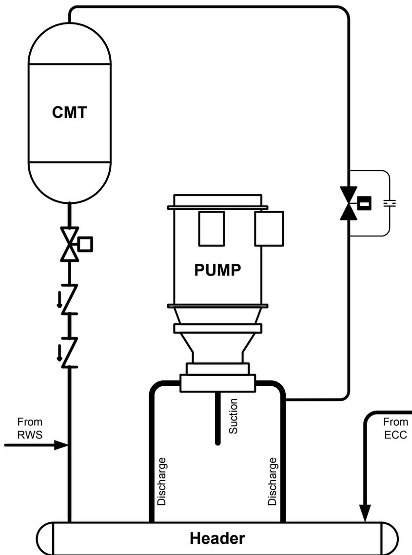
**Figure 3 ACR-1000 Core Make-Up Tank Configuration**
