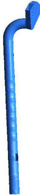
Fig. 1 An inlet nozzle assembly of the CANDU moderator circulation system
