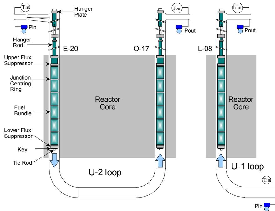
**Figure 1 Schematic Diagram of the Channel Configuration in U-1 and U-2 Loops**
