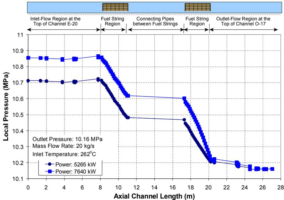
**Figure 3** Pressure Profiles along the U-2 Loop
