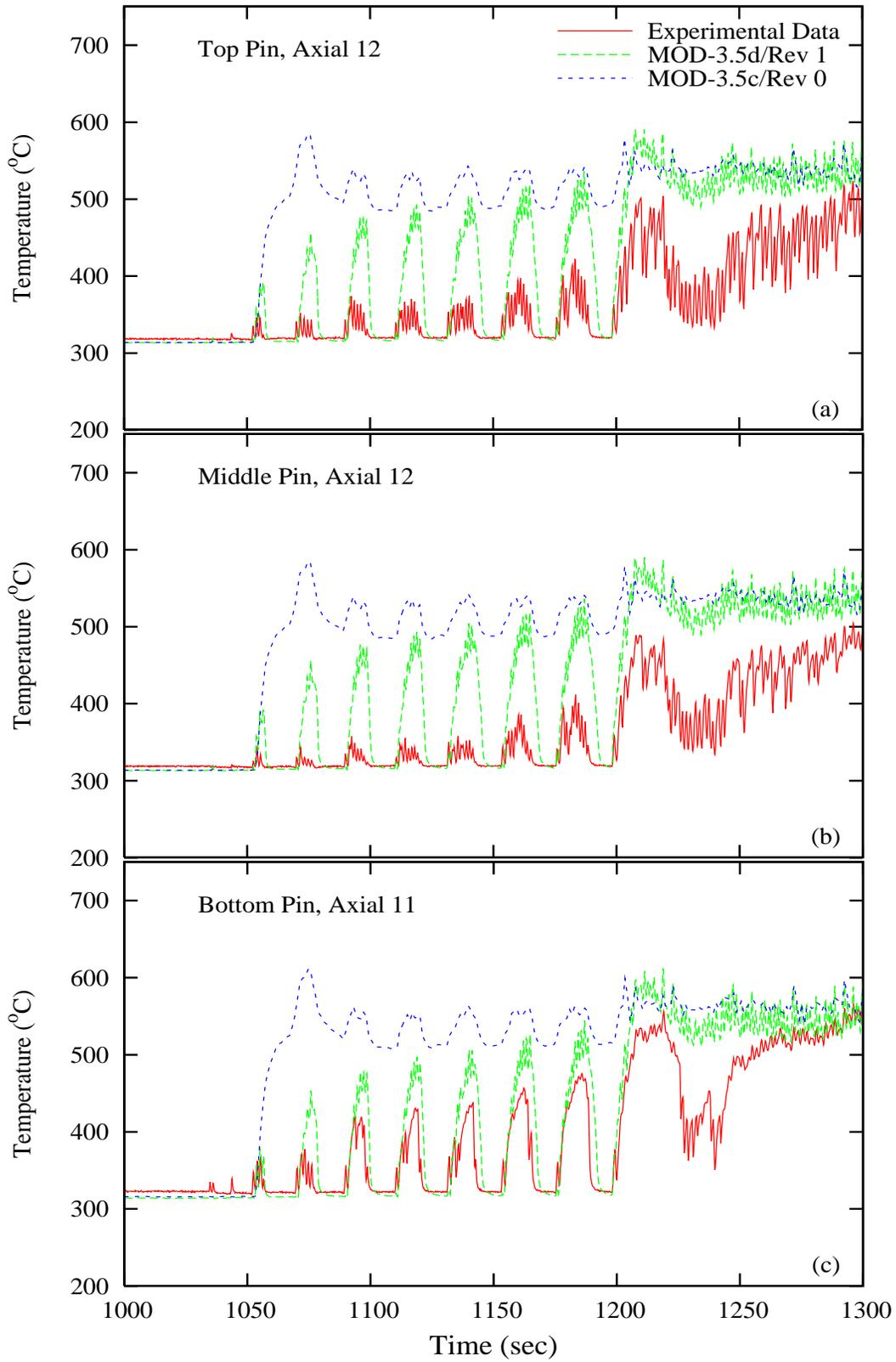
Figure 4: Measured and Predicted FES Temperatures in the (a) Top Pins (b) Middle Pins and (c) Bottom Pins Near the Outlet End of Heated Section 12
