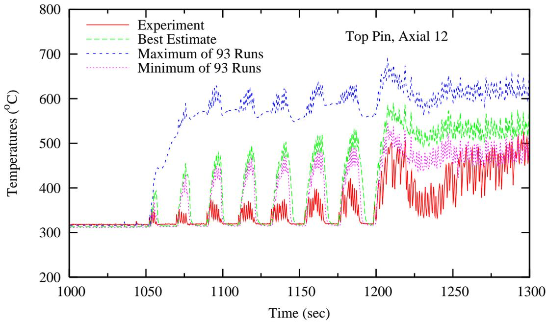
Figure 5: BE simulated and statistics FES Temperatures from 93 Simulations
