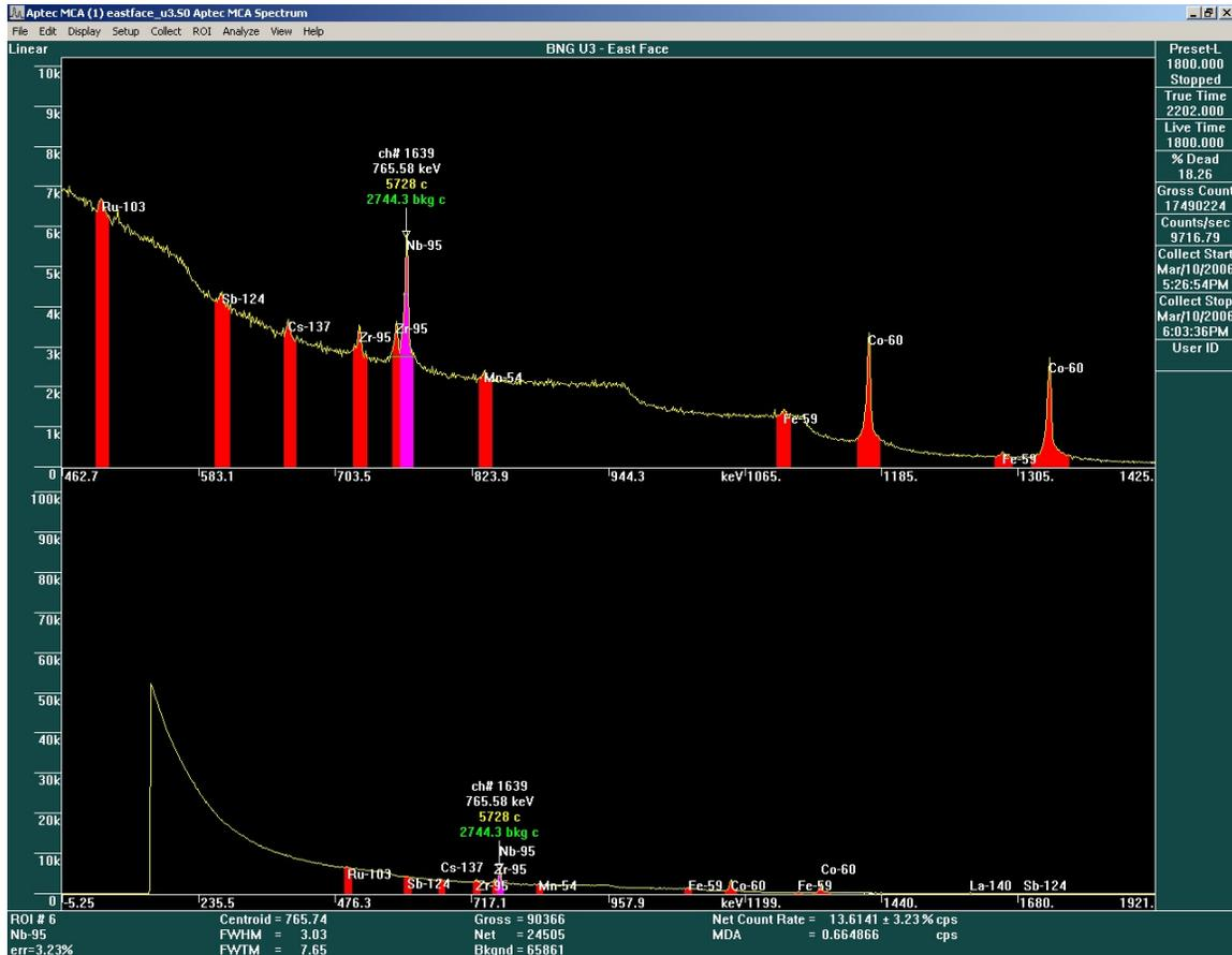
**Figure 1: Typical Reactor Face Spectrum Obtained Using a Germanium Detector System**
