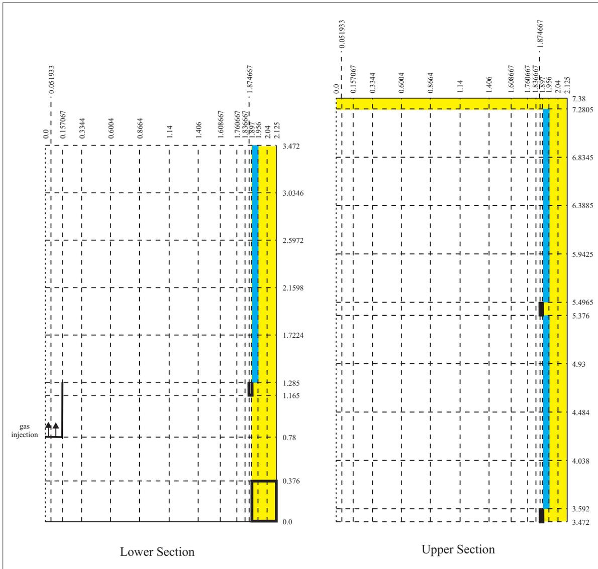
Figure 2: GOTHIC Model Nodalization of the MISTRA Facility (dimensions in m)
