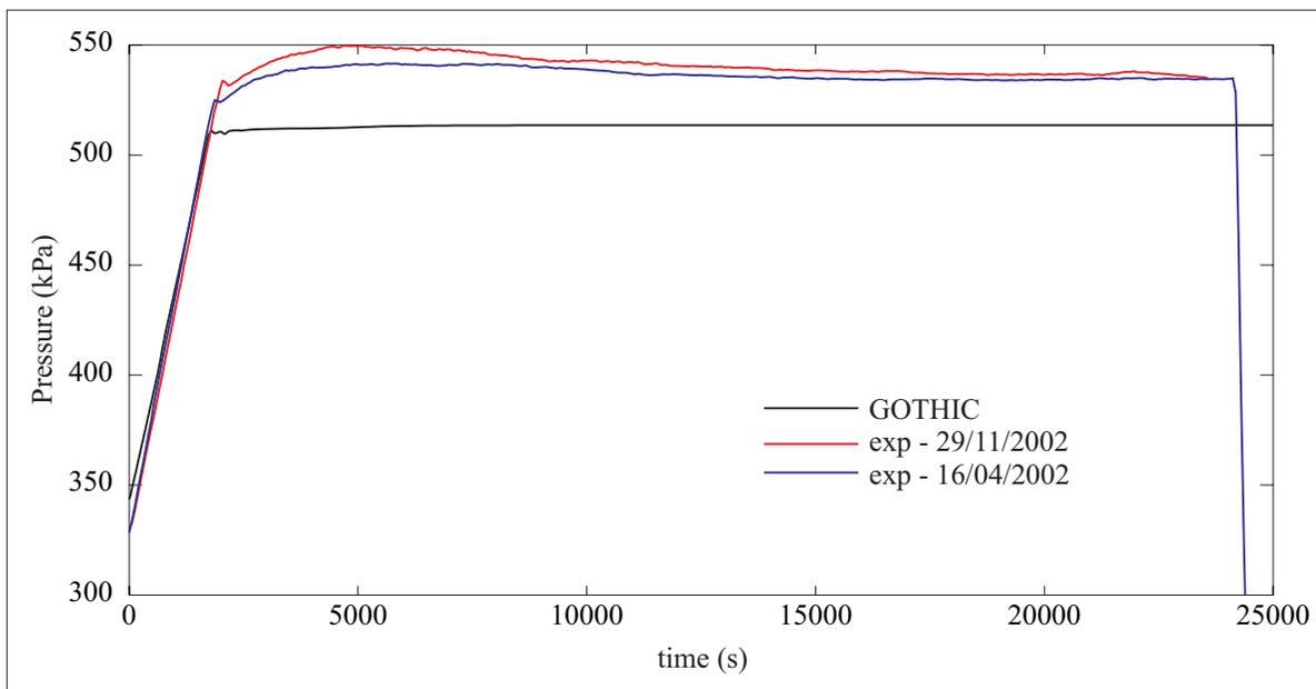
Figure 4: Pressure (Absolute) Transient After Start of Helium Injection
