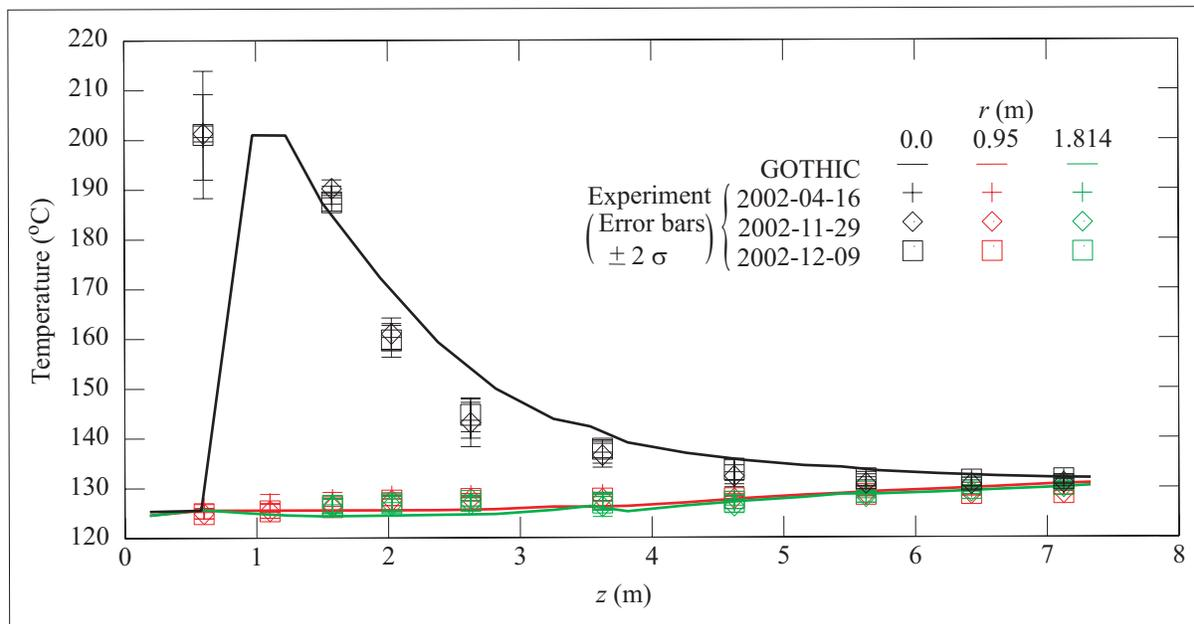
Figure 7: Steady State 2 Vertical Temperatures Profiles (along  $r = 0.0, 0.95$  and  $1.814$  m)
