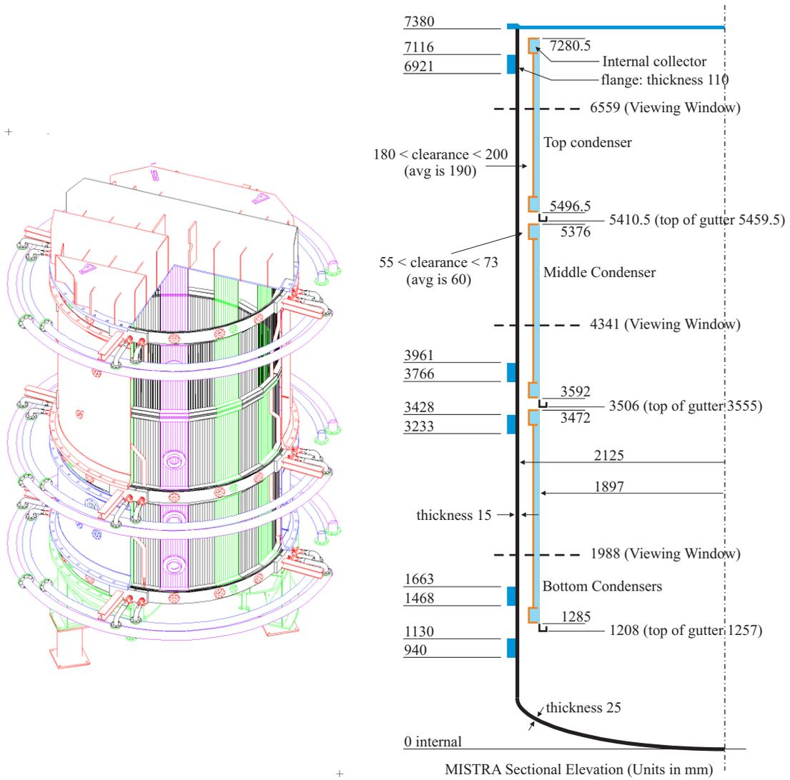
Figure 1: MISTRA Cut-out View and Elevation Cross-Section (dimensions are in mm)
