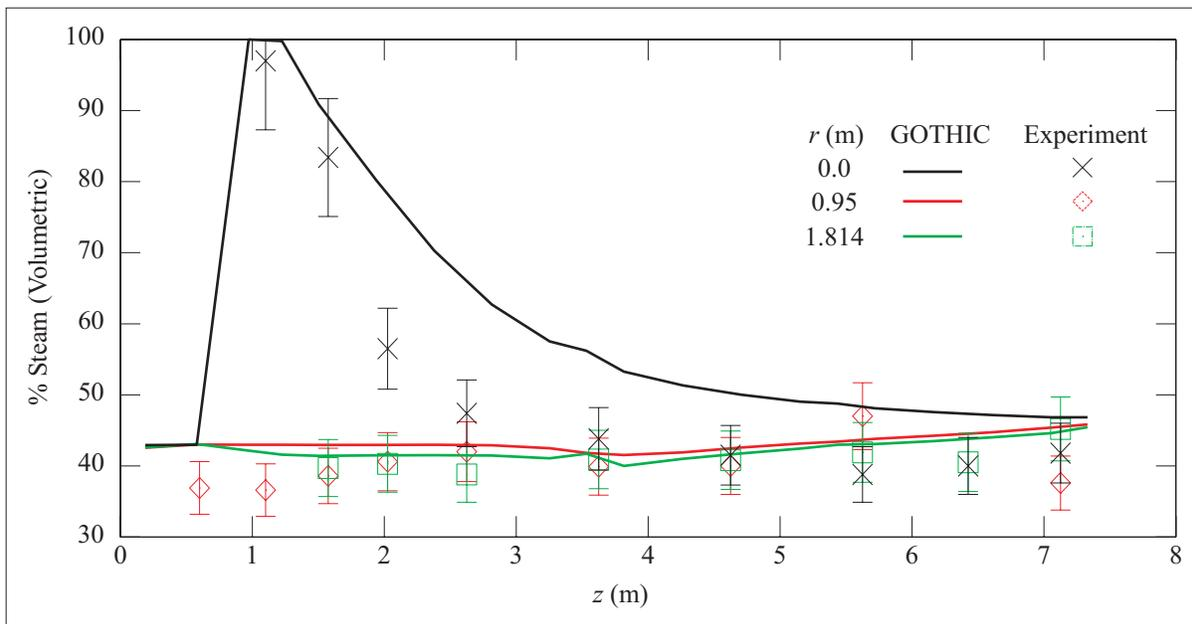
Figure 9: Steady State 2 Vertical Steam Concentration Profiles (along  $r = 0.0, 0.95$  and  $1.814$  m)
