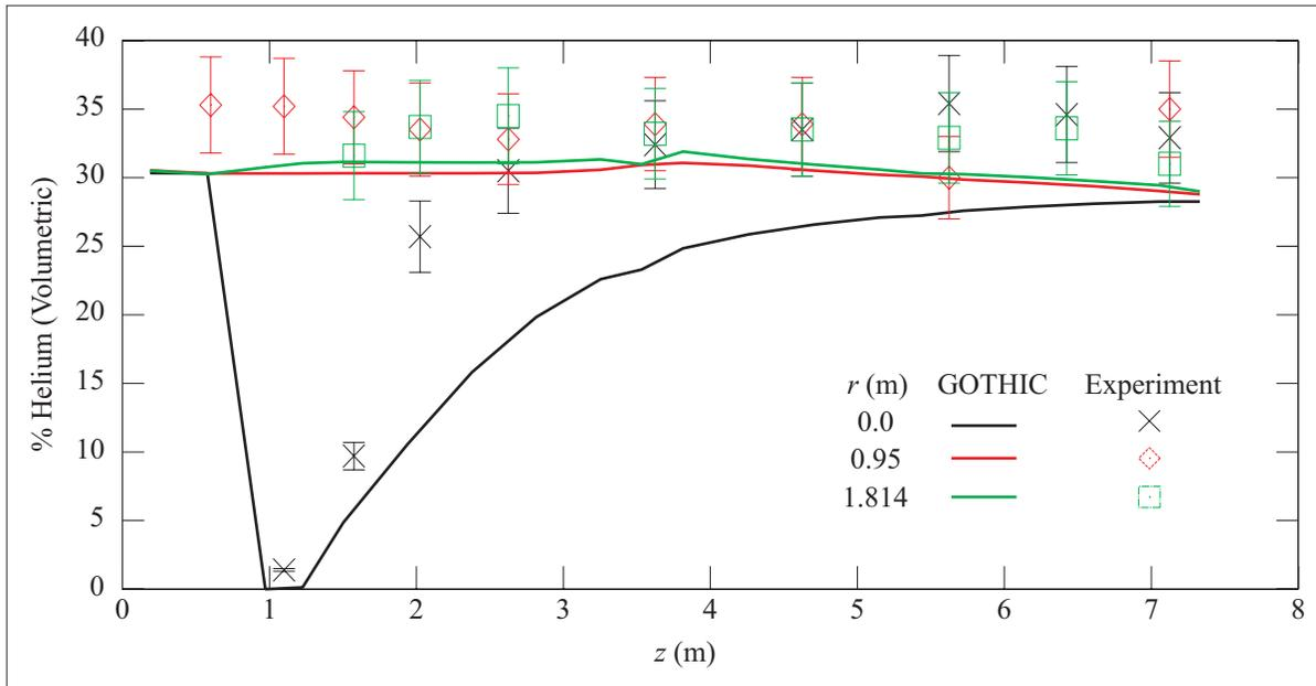
Figure 10: Steady State 2 Vertical Helium Concentration Profiles (along  $r = 0.0, 0.95$  and  $1.814$  m)
