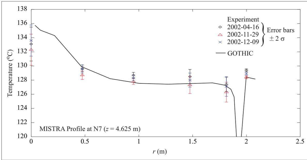
Figure 8: Steady State 2 Radial Temperatures Profiles at Mid Level ( $z = 4.625$  m)
