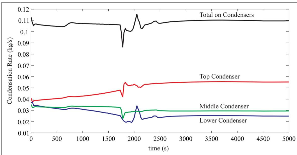
Figure 5: Condensation Rates Predicted by GOTHIC After Start of Helium Injection
