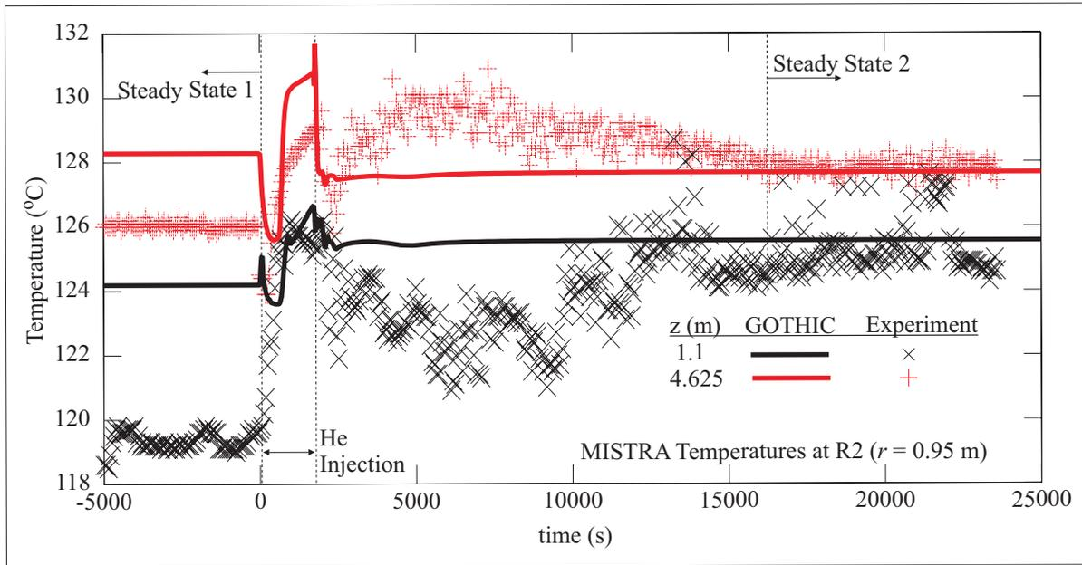
Figure 6: Transient Temperature at  $r = 0.95$  m and  $z = 1.1$  and  $4.625$  m
