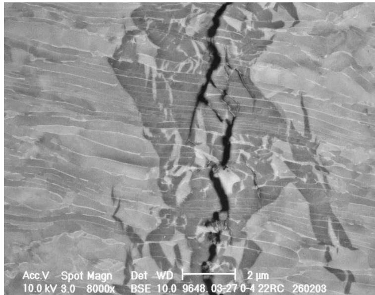
**Figure 1. SEM (Scanning Electron Microscope) micrograph of notch-tip hydrided region in an un-irradiated tube material,  $K_{EFF} = 12 \text{ MPa}\sqrt{m}$ , 22 ratcheting cycles.**
