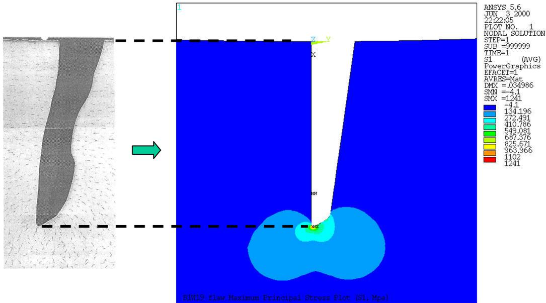
**Figure 3. Metallograph and finite element stress analysis of an ex-service debris fretting flaw for DHC initiation evaluation.**
