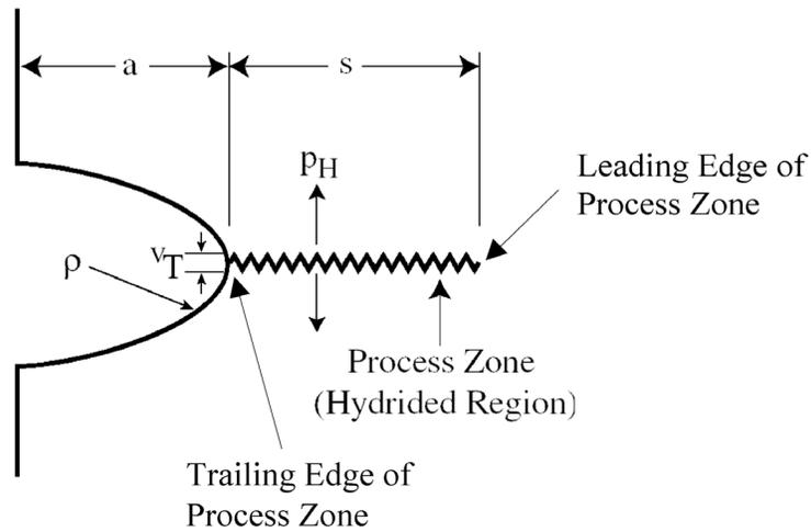
**Figure 4. Process Zone at a Flaw Tip**
