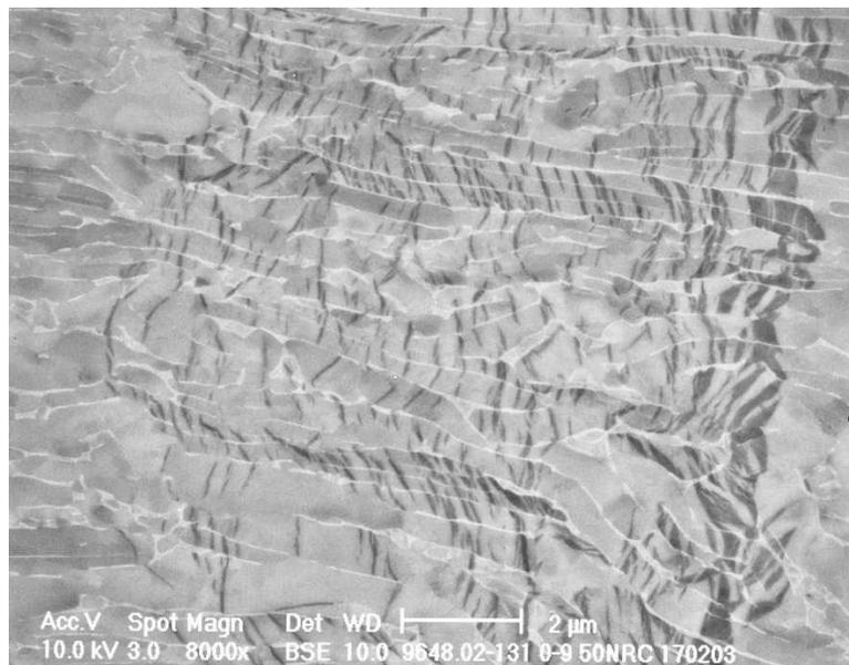
**Figure 2. SEM (Scanning Electron Microscope) micrograph of notch-tip hydrided region in an un-irradiated tube material,  $K_{EFF} = 12 \text{ MPa}\sqrt{m}$ , 50 non-ratcheting cycles.**
