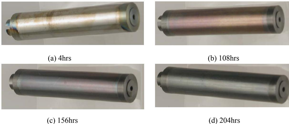
Figure 9. The oxidation of creep capsules heated in argon at 623K (hoop stress=300MPa)
