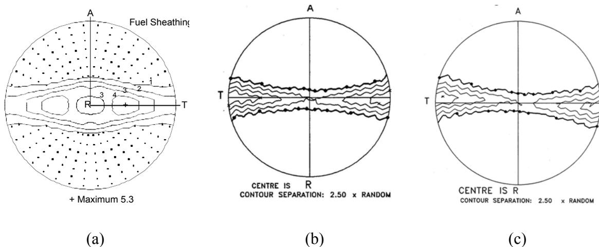
Figure 1. (0002) pole figure of (a) FS (b) MPT63 and (c) MPT66
