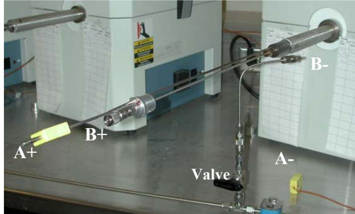
Figure 7. Argon gas protection assembly
