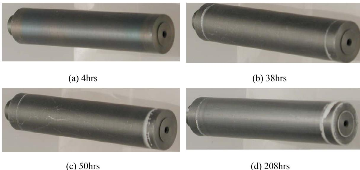
Figure 5. The oxidation of creep capsules heated in air at 623K (hoop stress=300MPa)
