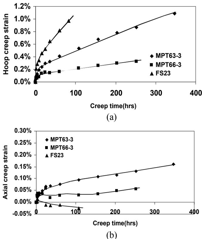
Figure 11. Creep time vs. strain (a) hoop (transverse) (b) axial at 623K
