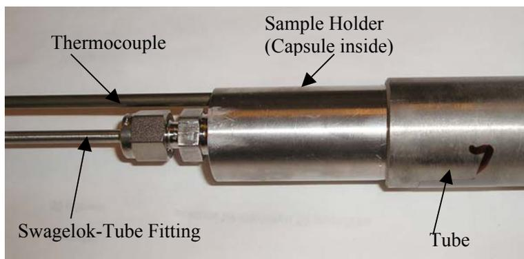
Figure 6. The creep sample holder for argon gas protection
