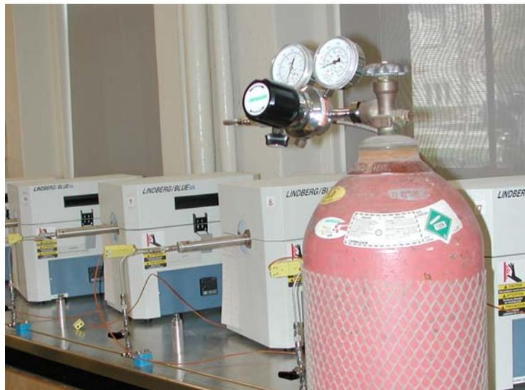
Figure 8. Overview argon gas protect system for thermal creep
