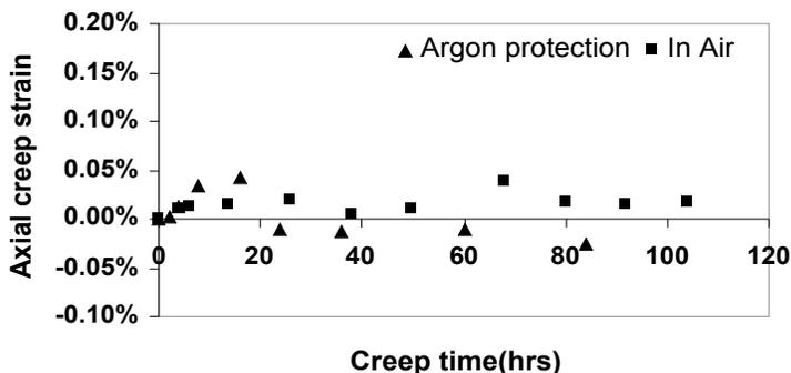
Figure 10. Axial creep strains vs. time under the hoop stress of 300MPa at 623K in Argon /Air
