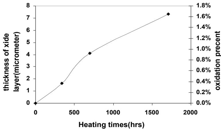
Figure 3. Heating time vs. oxidation percent at 673K in air heating atmosphere
