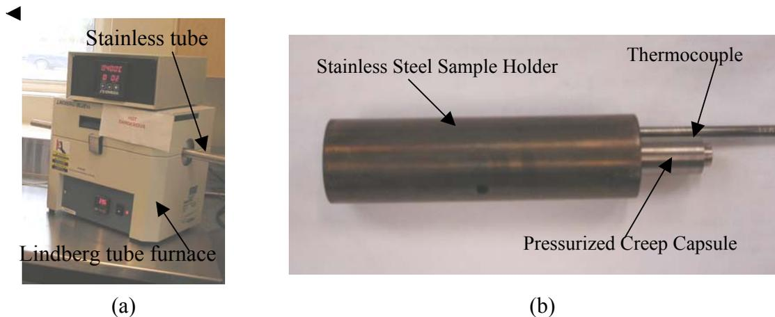
Figure 4. Lindberg tube furnace and sample holder for air atmosphere heating
