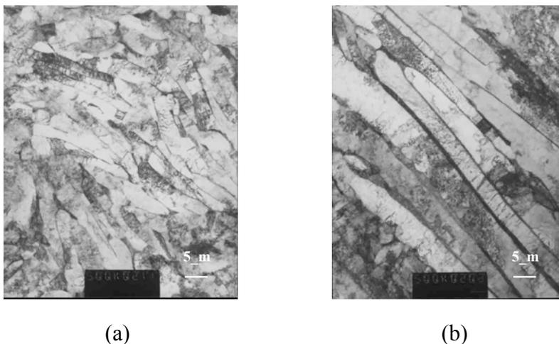
Figure 2. TEM microstructure (a) MPT63 and (b) MPT66
