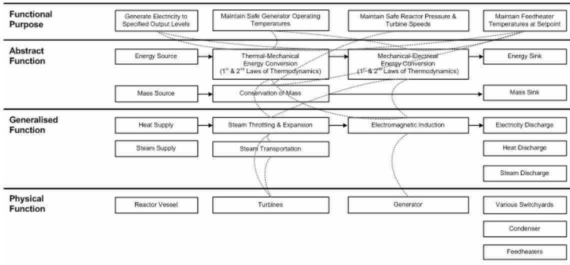
Figure 2: Abstraction Hierarchy at Part-Whole System Level [9]
