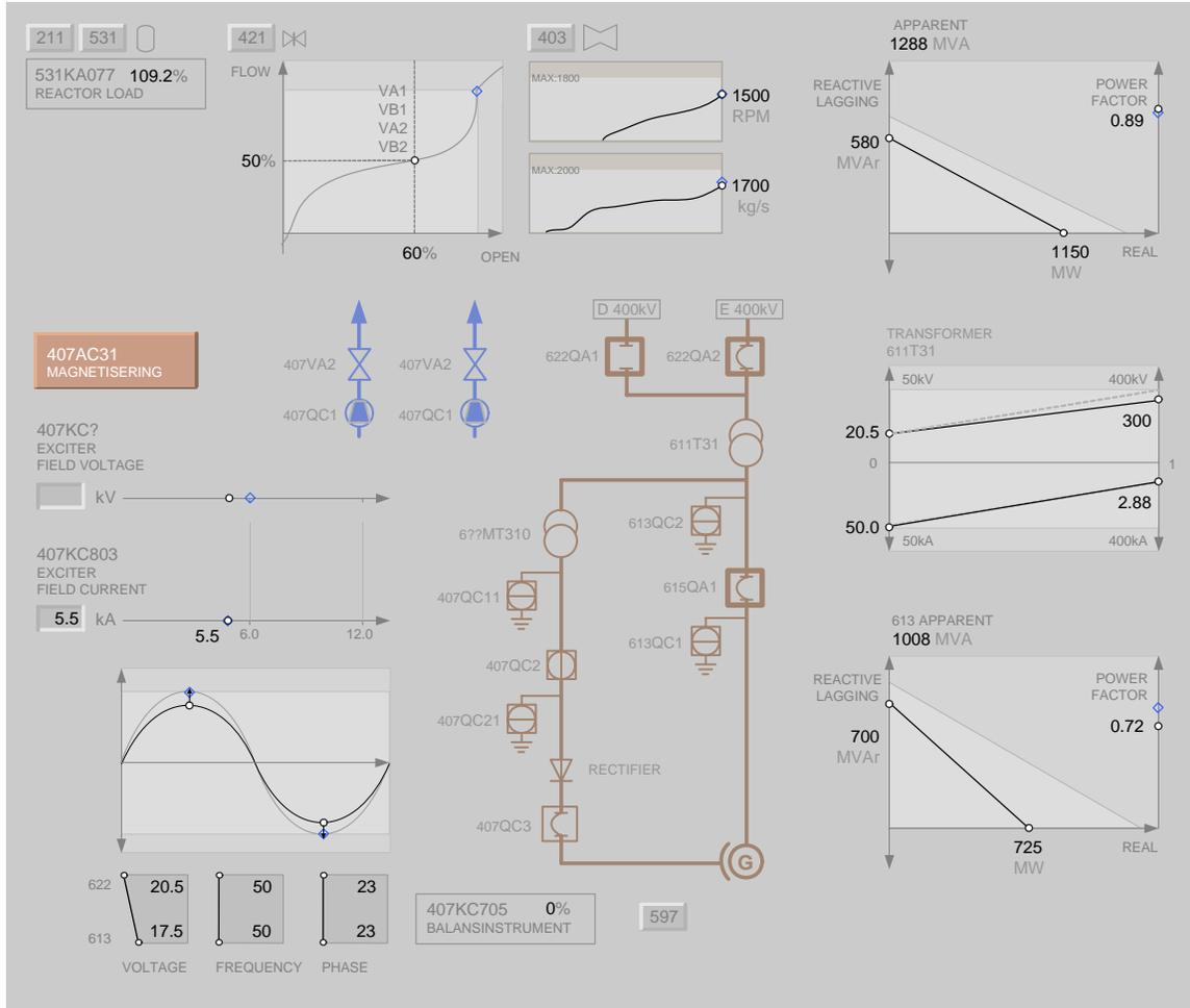
Figure 8: EID Graphical Display of the Generator Subsystem
