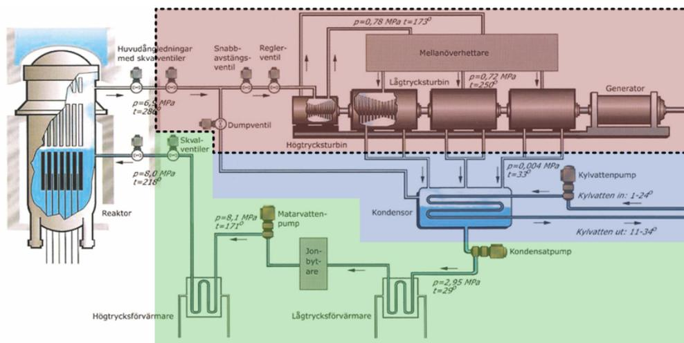
Figure 1: Turbine-Generator, Condenser, and Feedwater System Boundaries
