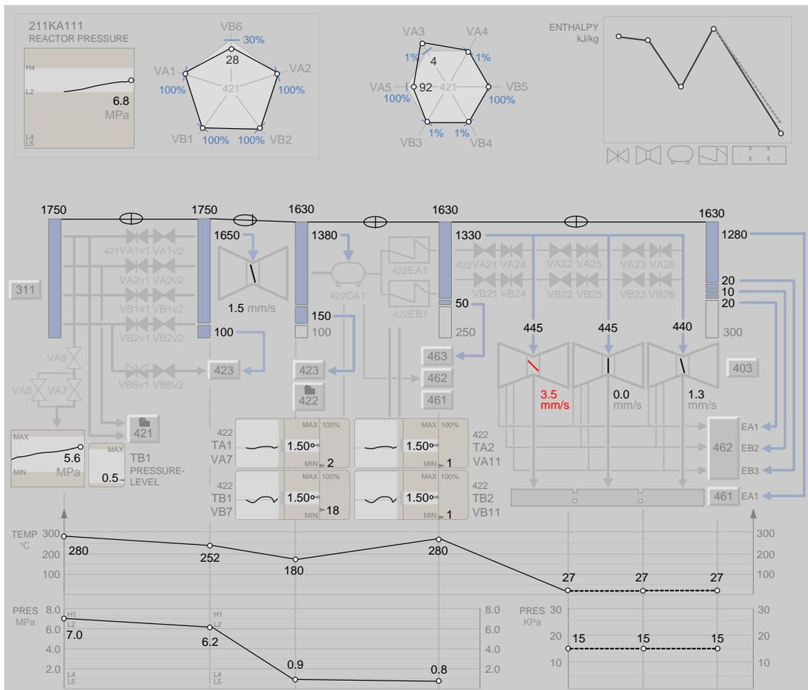
Figure 7: EID Graphical Display of the Turbine Subsystem
