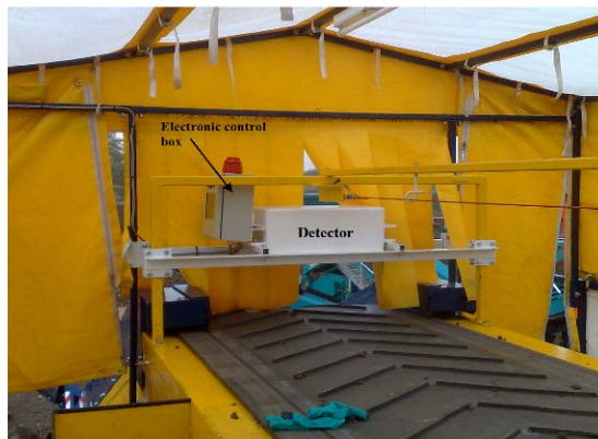
Figure 2 Monitoring Area of the Sorter Conveyor
