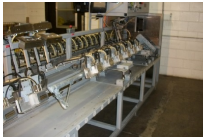
Figure 5, Third Generation – pipe is rotated in front of detector
