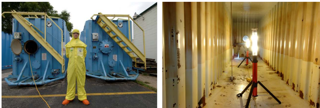
Figure 15 Frack Tank Decon and release for unrestricted use
