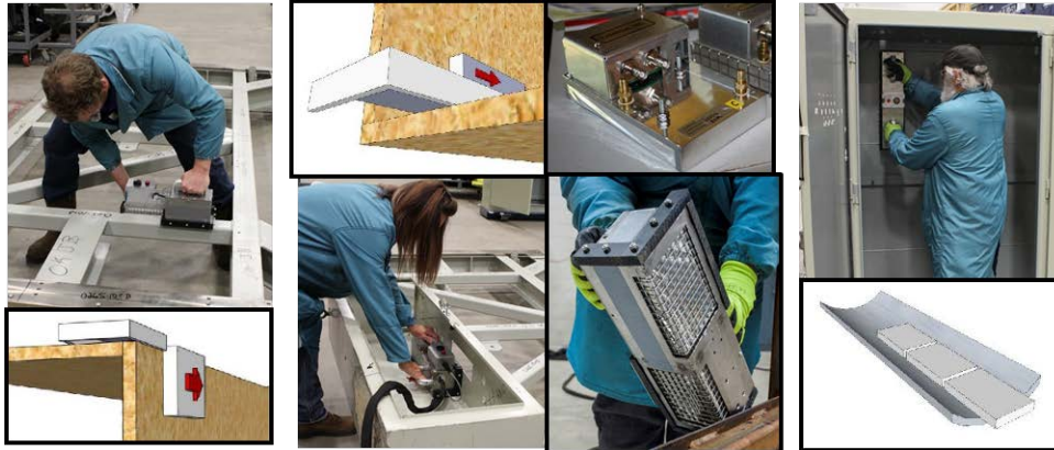
Figure 8 MJM Jigs, from left to right, outside corner, inside corner, 3 detector flat
