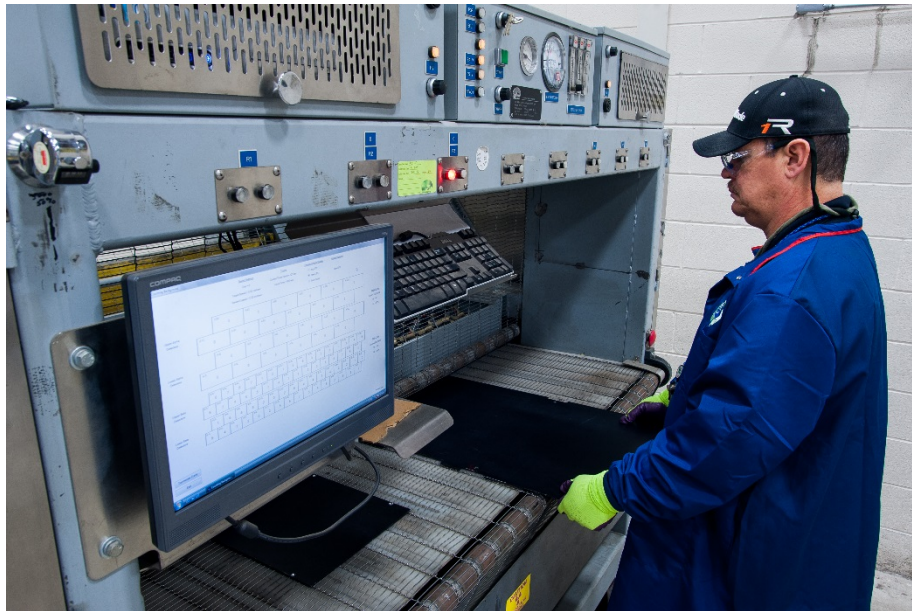
Figure 1 ABALM, 24 each 1200cm 2 Alpha Detectors, and 62 each 100cm 2 Beta/Gamma detectors
