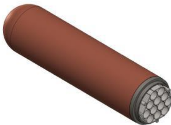
Figure 2: Copper Coated Used Fuel Container for CANDU Used Fuel proposed by the NWMO (48 bundle capacity).
