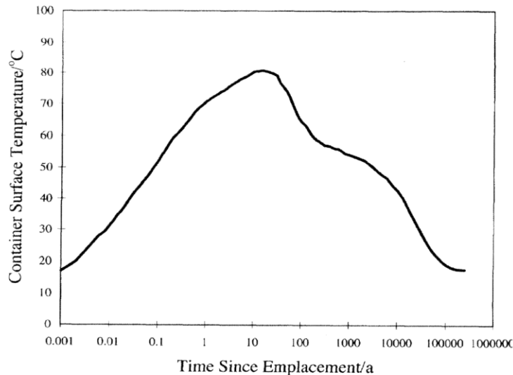
Figure 3: Predicted Variation of the Used Fuel Container Surface Temperature with Time for the In-Room DGR
