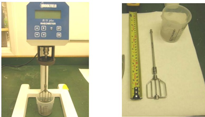
Figure 1 Rheometer and Paddle Used for MKP Slurry Mixing and Viscosity Measurement.
