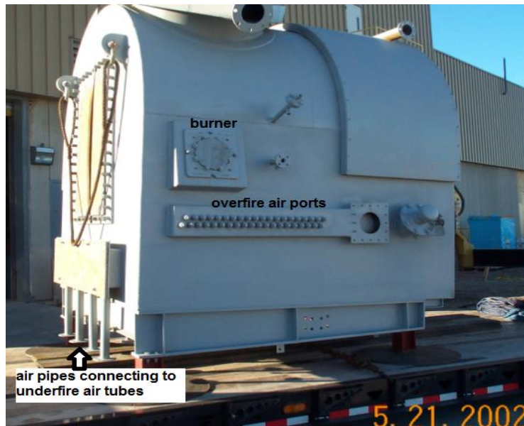
Figure 9: primary chamber 2002 being transported to site
