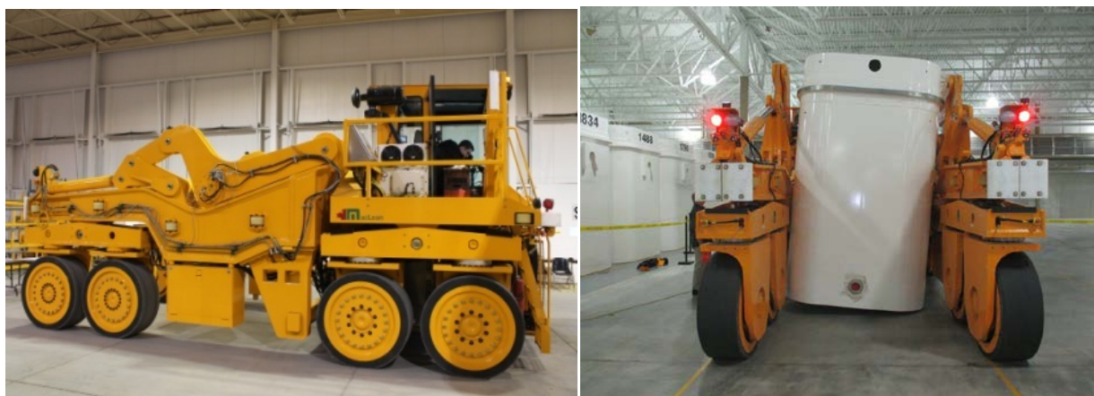
Figure 3 (a) Gen4 Transporter and (b) uneven lifting incident
