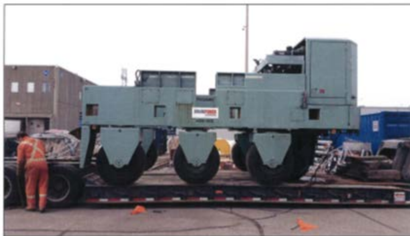
Figure 7 Body of Hammant with cab and lift structure removed ready for transport
