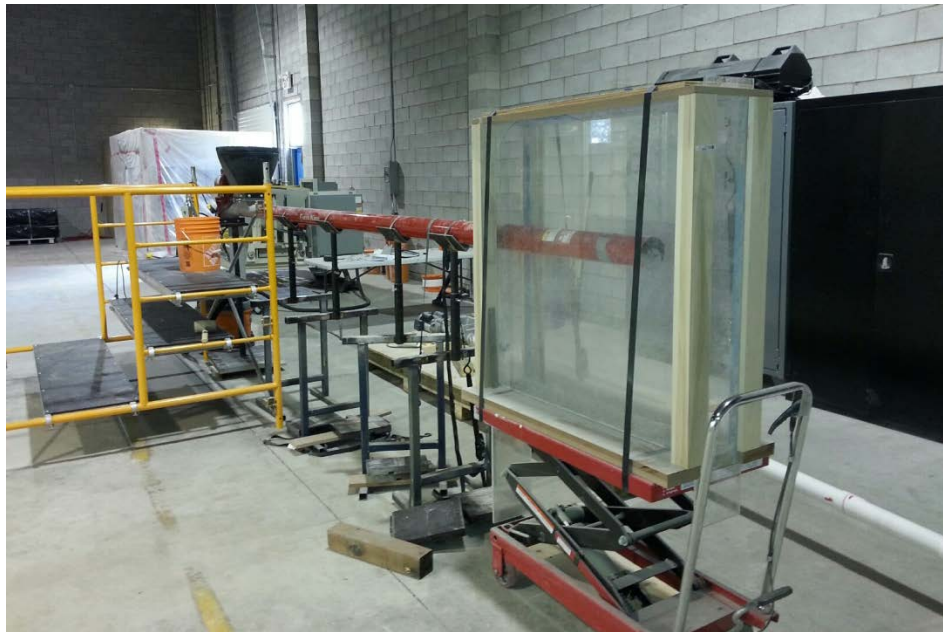
Figure 3 Photograph of utility screw conveyor and small scale test frame
