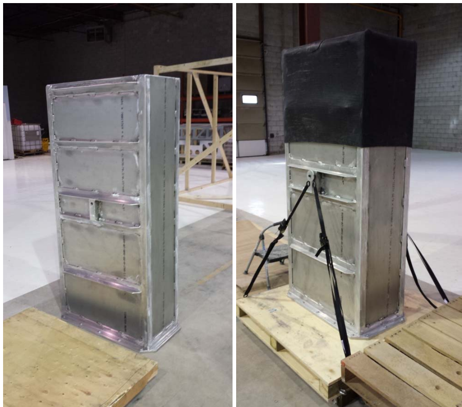
Figure 1 – Quarter Scale Container (left) and with Isostatic Bag (right)
