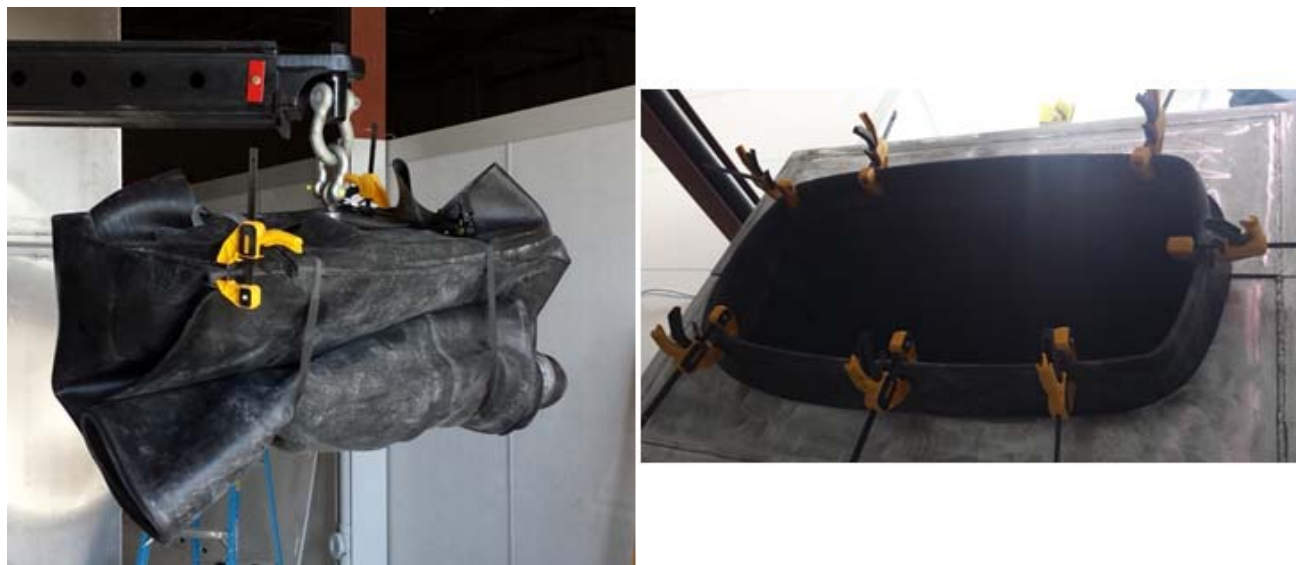
Figure 3 - Isostatic Bag rolled for installation (left), Bag secured over Vacuum Can (right) prior to bentonite loading for the full scale blocks
