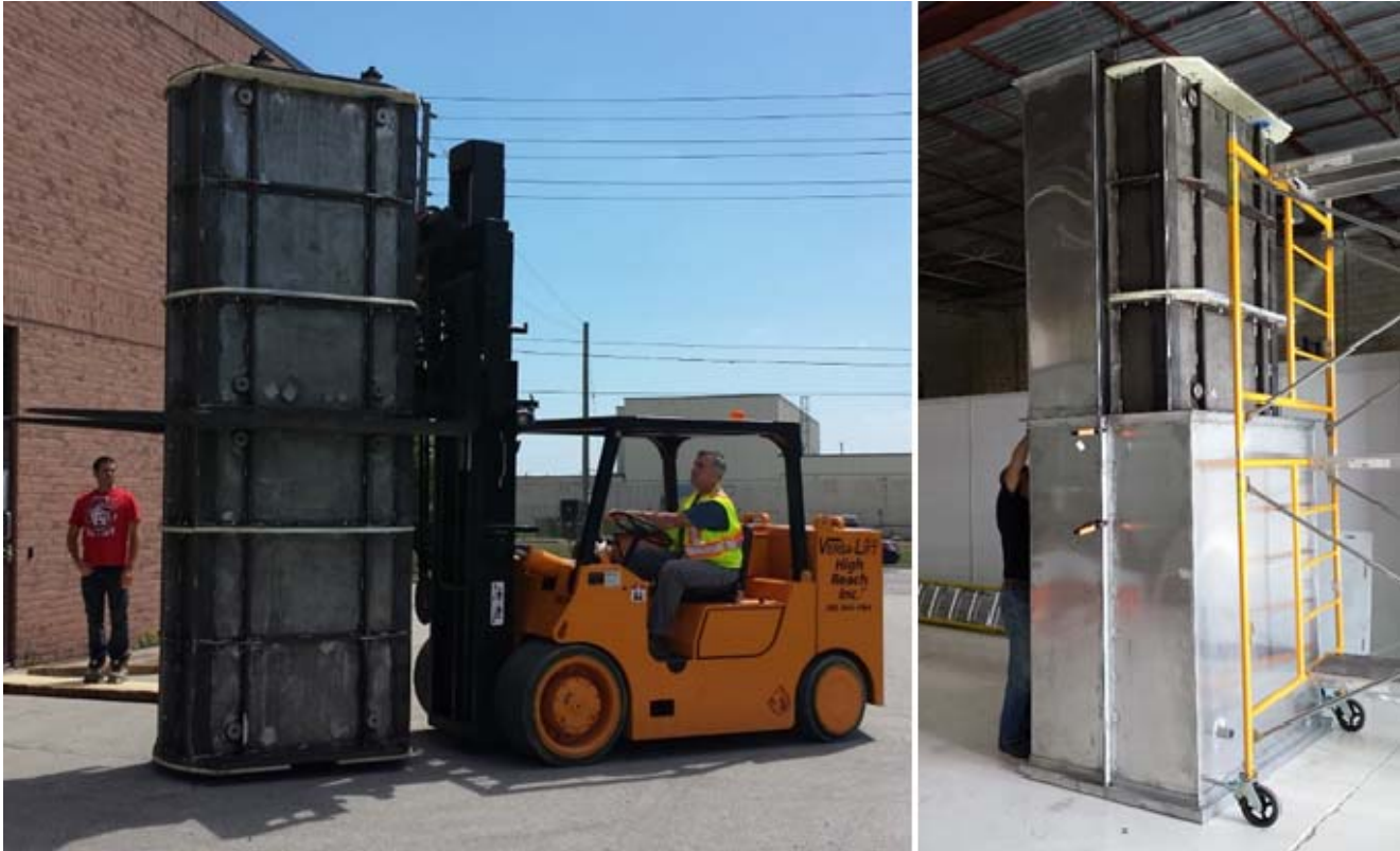
Figure 2 – Full-size Block Isostatic Container (left), Vacuum Can Assembly (right)
