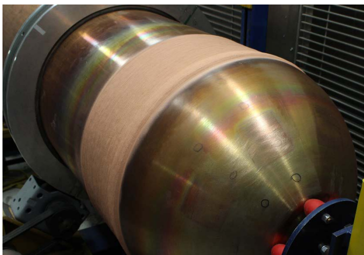
Figure 6: Prototype cold-spray coated container coated on the weld zone using cold spray.
