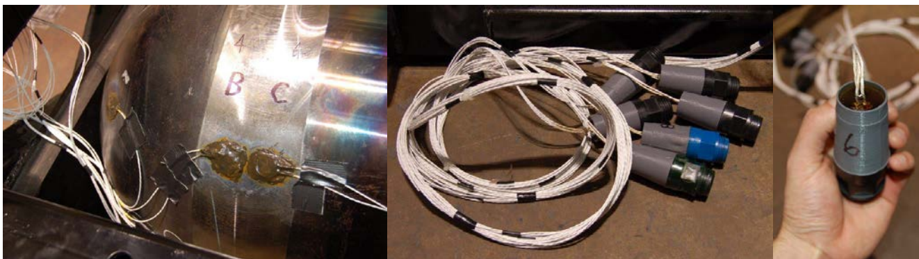
Figure 5 Strain gauges potted onto the Mark II Used Fuel Container prototype with water proof through-wall connectors
