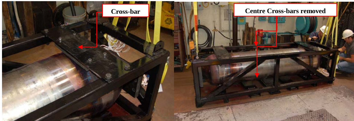
Figure 4 Used Fuel Container fixture configured for testing
