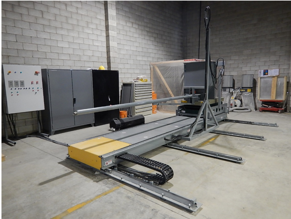
Figure 11: Gapfill Auger Delivery Platform
