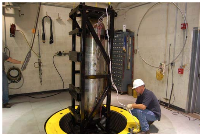
Figure 9: UFC Pressure Test
