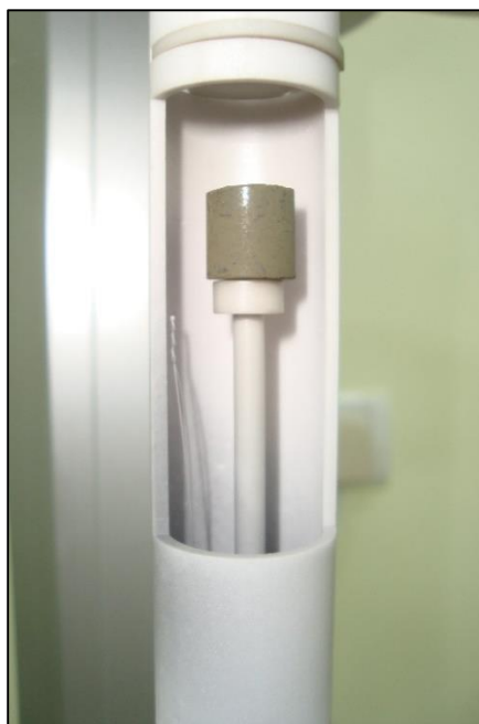
Figure 2 Actual Image of Sample mounted in a dilatometer
