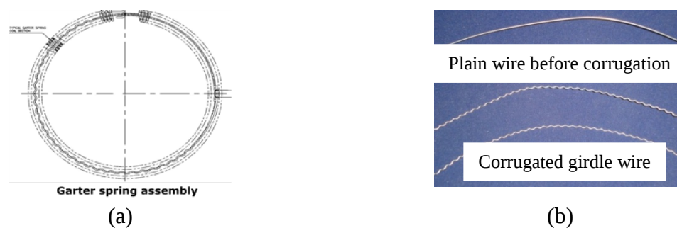
Figure 1 (a) Garter spring assembly for 700 MWe PHWRs and (b) Corrugated girdle wire.
