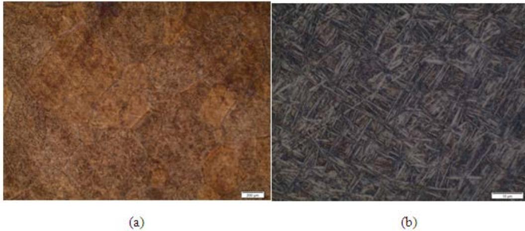
Figure 2[a-b] Optical micrographs of Zr-2.5%Nb-0.5%Cu extruded and \beta -quenched billet at 50x and 1000x respectively.
