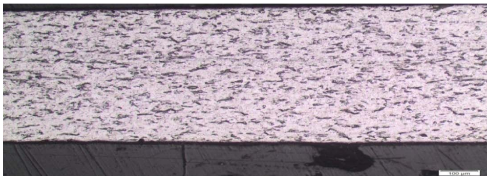
Figure 9 Optical micrographs showing hydride platelets oriented in axial direction of along the axis of annealed Zirconium alloy-4 plain girdle wire artificially hydrogen charged.
